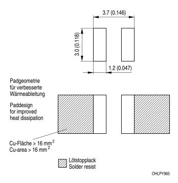
For superior solder joint connectivity results we recommend soldering under standard nitrogen atmosphere.
