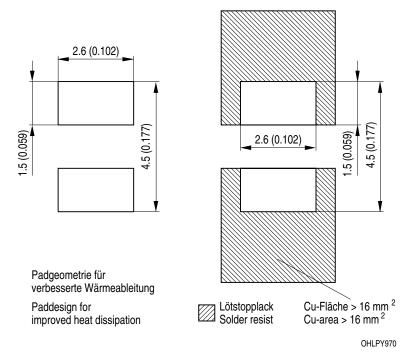
For superior solder joint connectivity results we recommend soldering under standard nitrogen atmosphere. Package not suitable for ultra sonic cleaning.
