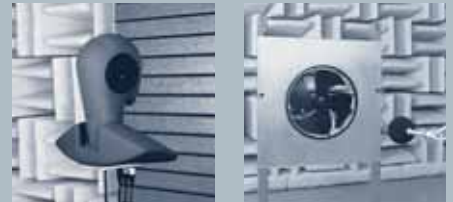
Room for precision noise measuring
