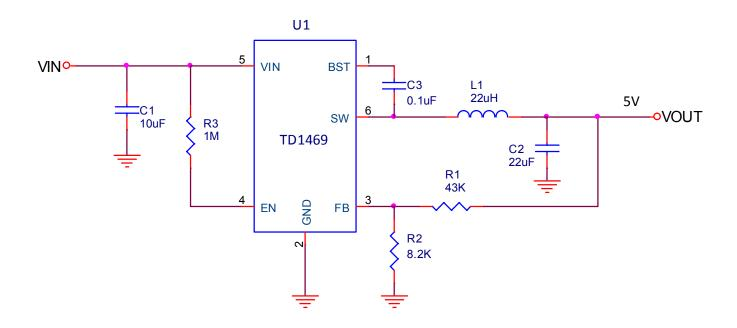
$$V_{OUT} = V_{REF}(1 + \frac{R1}{R2})$$
