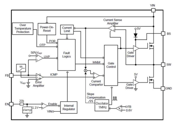
Figure 1 Function Block Diagram of TD1469
