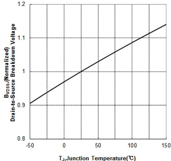
Figure 11 Typical Breakdown Voltage vs Junction Temperature
