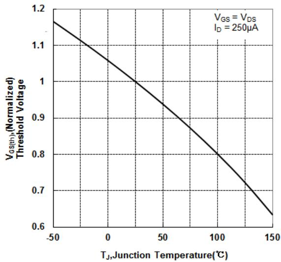
Figure 10 Typical Threshold Voltage vs Junction Temperature
