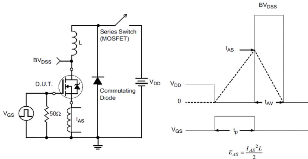
**Figure20.**Unclamped Inductive Switching Test Circuit
