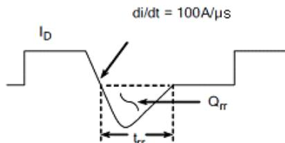
**Figure 19.** Diode Reverse Recovery Waveform
