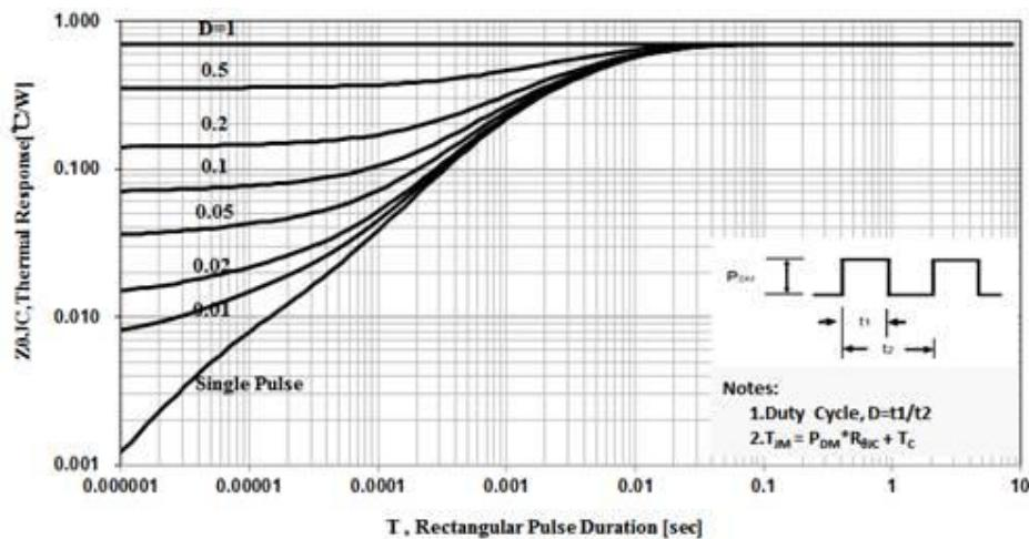
Figure 5 Maximum Effective Thermal Impedance , Junction to Case
