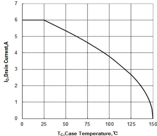
Figure 3 Maximum Continuous Drain Current vs Case Temperature
