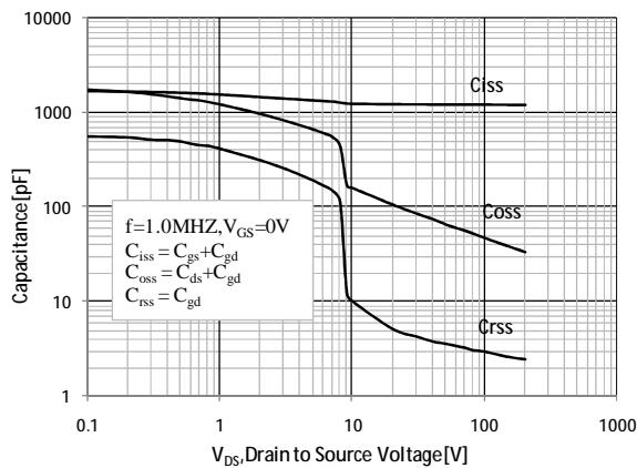
Figure 12 Typical Capacitance vs Drain to Source Voltage
