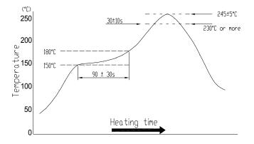
Temperature profile for reflow soldering
