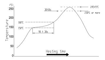
Temperature profile for reflow soldering
