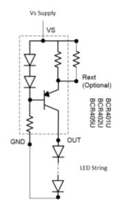
Figure 1 Typical Application Circuit for BCR40x LED Driver
