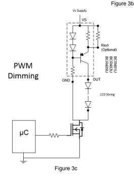
Figure 3a, 3b, & 3c. Application Circuits for LED Driver with PWM Dimming Functionality
