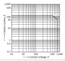
1-2.Max. switching capacity (DC resistive load)
