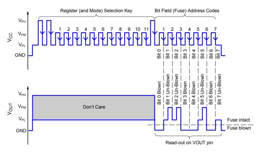
Figure 9. Read mode example. Pulse sequence for accessing the B<sub>OP</sub> Selection register (BOPSEL) and reading back the status of each of the eight bit fields. In this example, the code (blown fuses) is  $2^0 + 2^3 + 2^4 + 2^6 = 89$  (0101 1001). After each address pulse is sent, the voltage on the VOUT pin will be at GND for blown fuses and at V<sub>CC</sub> (at V<sub>PL</sub> or V<sub>PM</sub>) for un-blown fuses.
