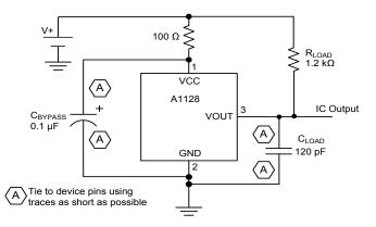
Figure 1. Typical Application Circuit
