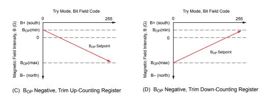
Figure 12. B<sub>OP</sub> profiles for each of the four B<sub>OP</sub> Selection virtual registers available in Try mode.
