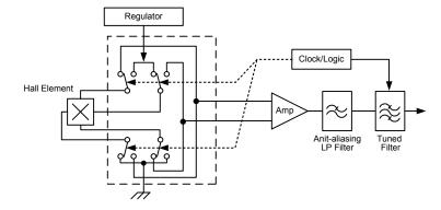
Figure 2. Concept of Chopper Stabilization Technique
