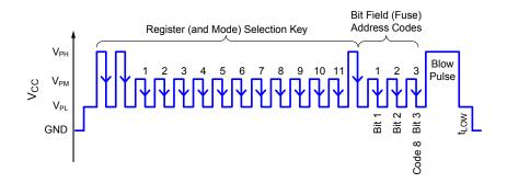
Figure 11. Example of Blow mode programming pulses applied to the VCC pin. In this example, the  $B_{OP}$  Magnitude Selection register (BOPSEL) is addressed to code 8 (bit 3, or 3  $V_{PM}$  pulses) and its value is permanently blown.
