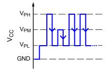
Figure 5. Example of Try mode register selection pulses, for the  ${\sf B}_{{\sf OP}}$  Negative Trim, Up-Counting register.
