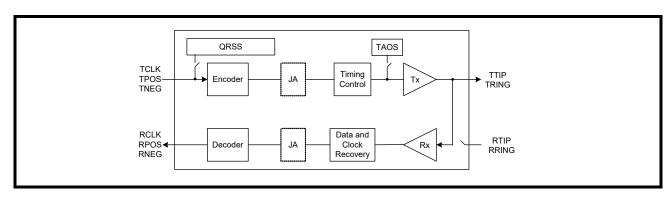
**Note:** The transmit diagnostic features such as TAOS and QRSS take priority over the transmit input data at TCLK/TPOS/TNEG.
