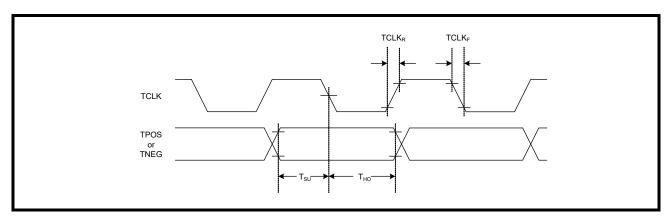
FIGURE 18. TRANSMIT DATA SAMPLED ON RISING EDGE OF TCLK
