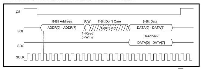
**Note:** For applications without a free running SCLK, a minimum of 1 SCLK pulse must be applied when  $\overline{\text{CS}}$  is "High", befrore pulling  $\overline{\text{CS}}$  "Low".
