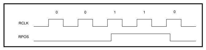
FIGURE 14. DUAL RAIL MODE WITH A FIXED REPEATING "0011" PATTERN
