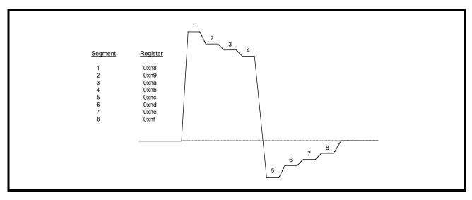
**Note:** By default, the arbitrary segments are programmed to 0x00h. The transmitter outputs will result in an all zero pattern to the line interface.
