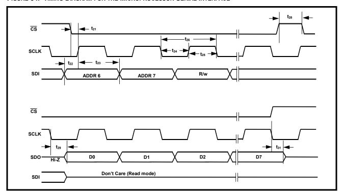
Table 12: Microprocessor Serial Interface Timings (  $T_A = 25^{\circ}C$ ,  $V_{DD} = 3.3V \pm 5\%$  and load = 10pF)
