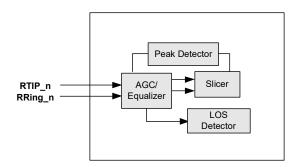
Figure 7: AGC and Equalizer Block Diagram
