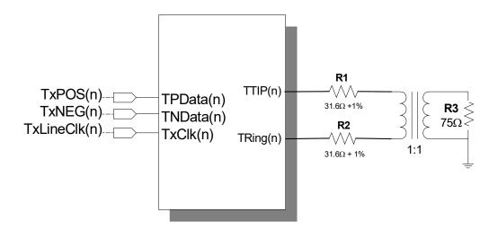
Figure 19: Transmit Pulse Shape Test Circuit
