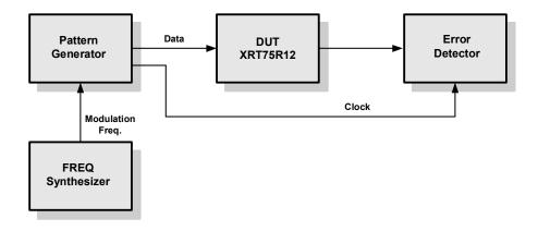
Figure 24: Jitter Tolerance Measurements
