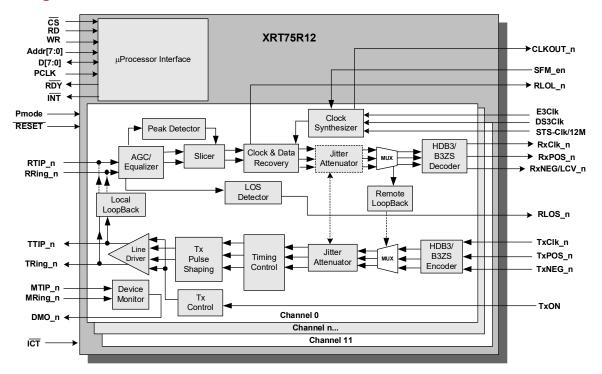
Figure 1: XRT75R12 Block Diagram
