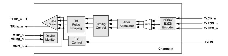
Figure 12: Transmit Path Block Diagram
