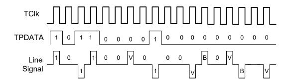
Figure 17: B3ZS Encoding Format
