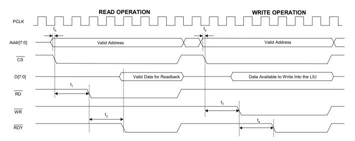
Figure 35: Synchronous µP Interface Signals During Programmed I/O Read and Write Operations
