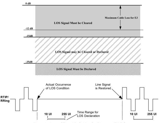
Figure 8: Loss of Signal Definition for E3 as per ITU-T G.775
