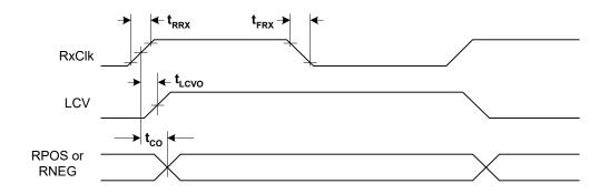
Figure 11: Receiver Data Output and Code Violation Timing
