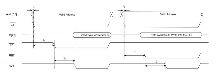
Figure 34: Asynchronous μP Interface Signals During Programmed I/O Read and Write Operations
