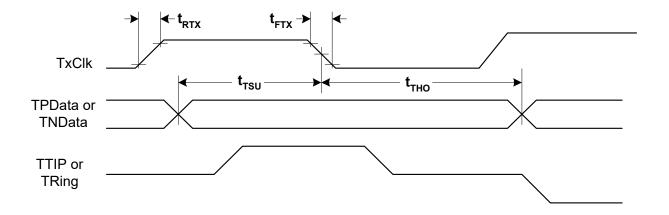
Figure 14: Transmitter Terminal Input Timing
