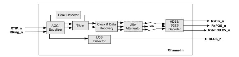
Figure 5: Receive Path Block Diagram
