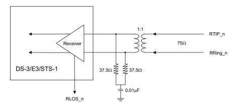
Figure 6: Receive Line Interface Connection
