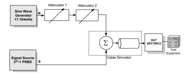
Figure 10: Interference Margin Test Set Up for E3
