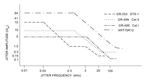
Figure 25: Input Jitter Tolerance for DS3 and STS-1
