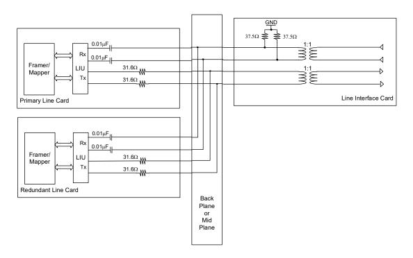
Figure 2: Network Redundancy Architecture
