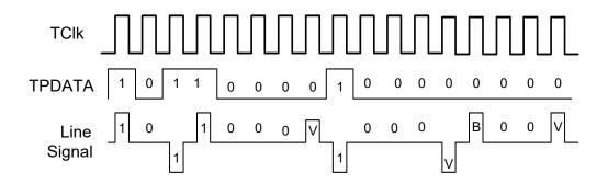
Figure 18: HDB3 Encoding Format
