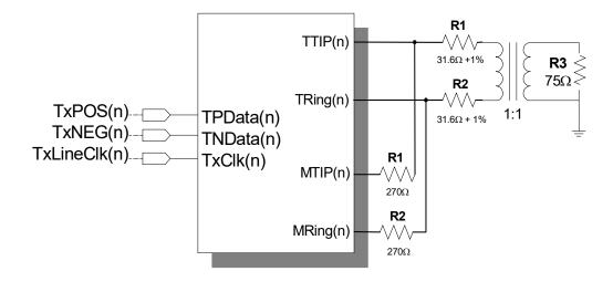
Figure 23: Transmit Driver Monitor Set Up
