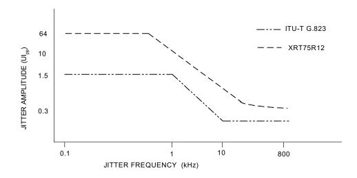
Figure 26: Input Jitter Tolerance for E3
