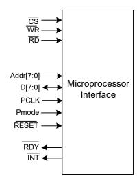
Figure 33: Simplified Block Diagram, Microprocessor Interface
