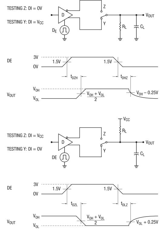
Figure 8. Driver Enable and Disable Timing Test Circuits and Timing Diagrams
