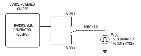
Figure 6. Transient Overvoltage Test Circuit
