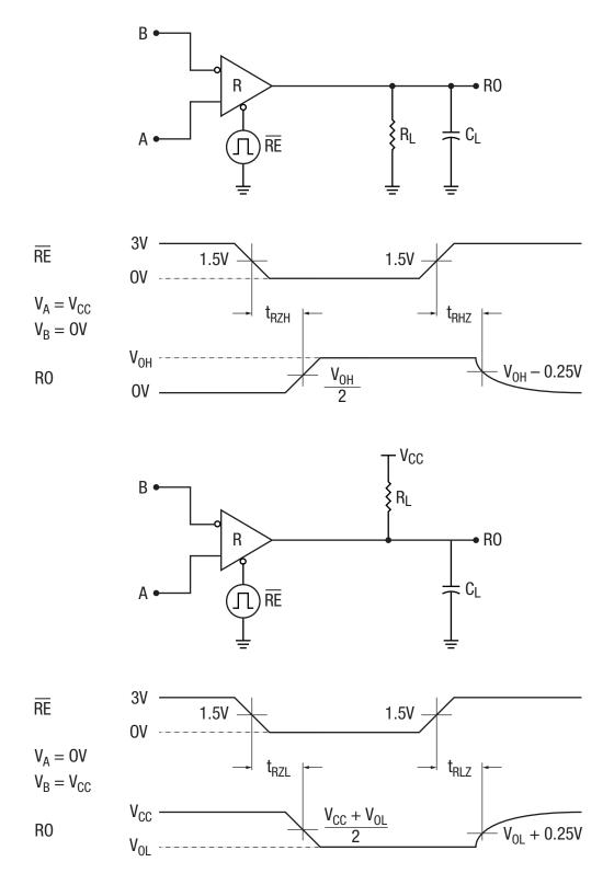
Figure 10. Receiver Enable and Disable Test Circuits and Timing Diagrams
