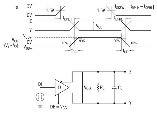
Figure 7. Driver Propagation Delay Test Circuit and Timing Diagram
