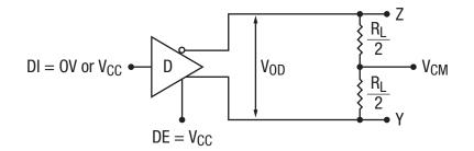
Figure 3. Differential Driver Output Voltage
