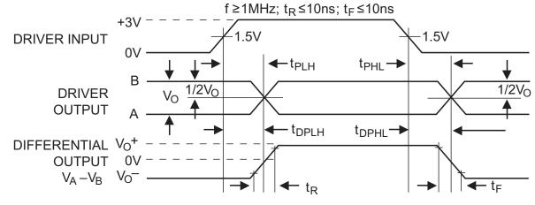
$t_{SKEW} = |t_{DPLH} - t_{DPHL}|$
