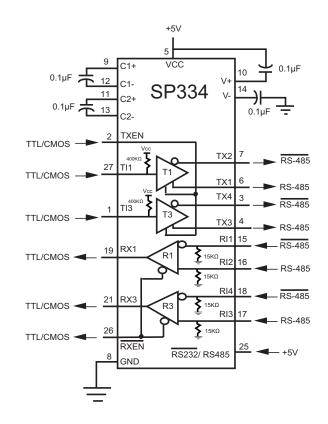
Figure 12. Typical Operating Circuits
