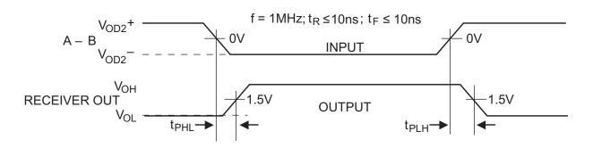
Figure 7. Receiver Propagation Delays
