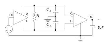
Figure 3. Driver / Receiver Timing Test Circuit
