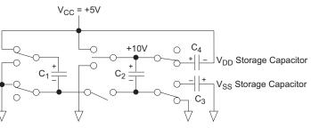
Figure 16. Charge Pump Phase 4
