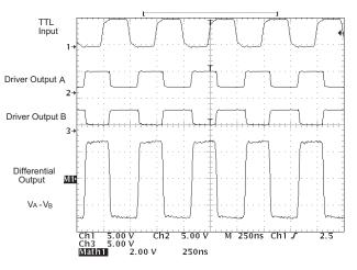
Figure 10. Typical RS-485 Driver Output
