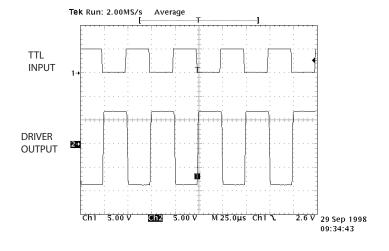
Figure 9. Typical RS-232 Driver Output
