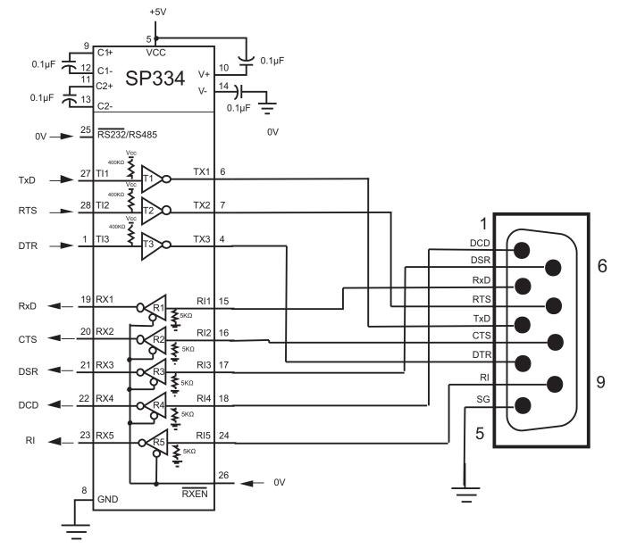
Figure 18. SP334 Configuration to a DB-9 Serial Port
