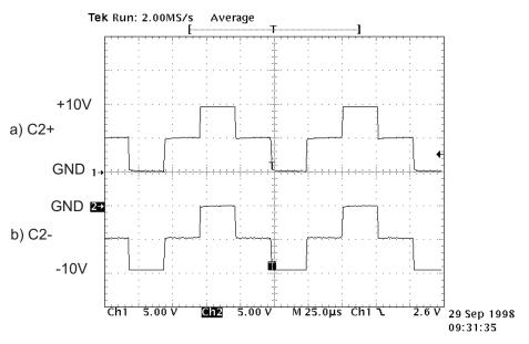
Figure 17. Charge Pump Waveforms
