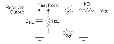
Figure 2. Receiver Timing Test Load Circuit
