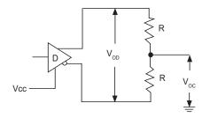
Figure 1. Driver DC Test Load Circuit
