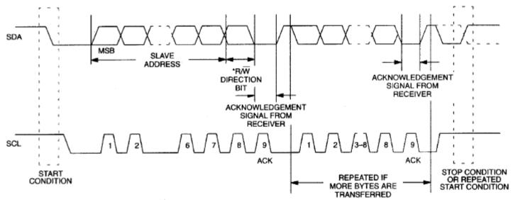
Depending upon the state of the  $R/\overline{W}$  bit, two types of data transfer are possible:
