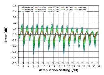
Figure 21. Step Accuracy vs Attenuator Setting [LSB = 1.00dB]
