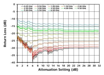
Figure 9. Output Return Loss vs Attenuator Setting
