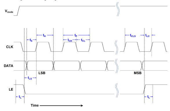
Table 10. SPI Timing Diagram Values for the Serial Mode
