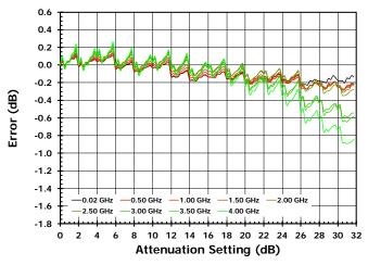
Figure 13. Absolute Accuracy vs Attenuator Setting [LSB = 0.50dB]
