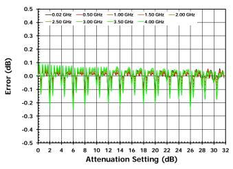
Figure 19. Step Accuracy vs Attenuator Setting [LSB = 0.50dB]
