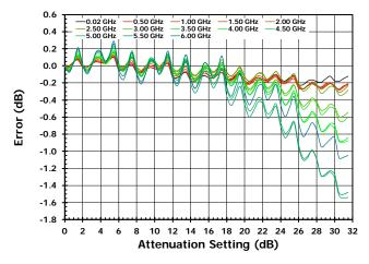
Figure 15. Absolute Accuracy vs Attenuator Setting [LSB = 1.00dB]
