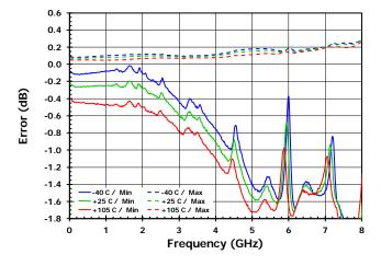
Figure 11. Absolute Accuracy vs Attenuator Setting [LSB = 0.25dB]
