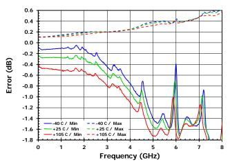
Figure 12. Worst Case Absolute Accuracy vs Frequency [LSB = 0.50dB]
