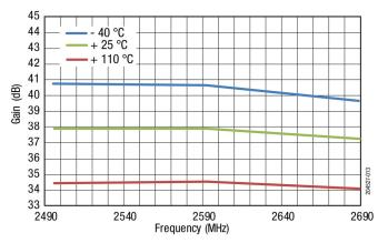
Figure 13. Small Signal Gain vs Frequency Across Temperature
