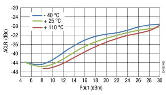
Figure 6. LTE 5x20 MHz ACLR1 vs Pout Across Temperature
