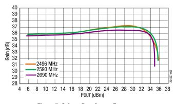
Figure 7. Gain vs Pout Across Frequency
