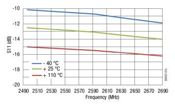
Figure 15. S11 vs Frequency Across Temperature (PIN = -20 dBm)
