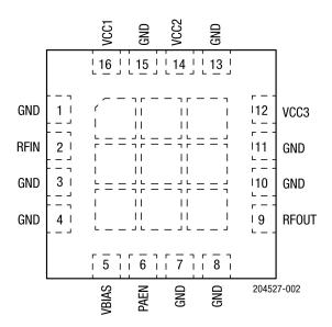
Figure 2. SKY66317-11 Pinout (Top View)
