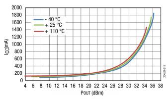
Figure 10. IOP vs Pout Across Temperature
