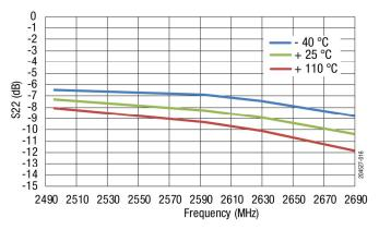
Figure 16. S22 vs Frequency Across Temperature (PIN = -20 dBm)
