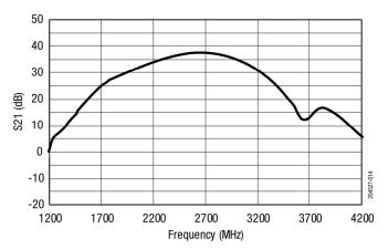
Figure 14. Wide-Band S21 vs Frequency
