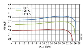
Figure 8. Gain vs Pout Across Temperature
