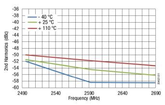
Figure 11. 2nd Harmonic @ +28 dBm (CW) vs Frequency Across Temperature
