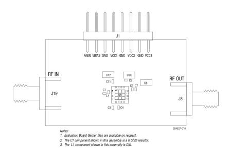
Figure 18. SKY66317-11 Evaluation Board Assembly Drawing
