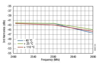
Figure 12. 3rd Harmonic @ +28 dBm (CW) vs Frequency Across Temperature
