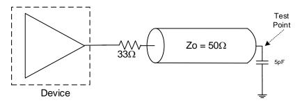
Figure 3. HCSL/LPHCSL Test Load
