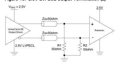
Figure 17. 2.5V LVPECL Output Termination (3)
