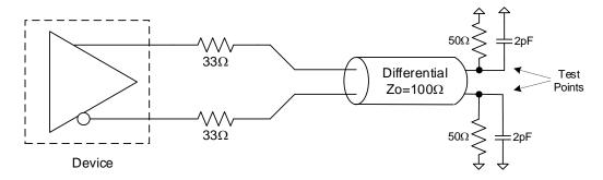
Figure 4. LVDS Test Load
