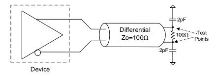
Figure 5. LVPECL Test Load
