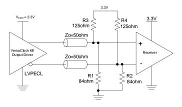
Figure 16. 2.5V LVPECL Output Termination (2)
