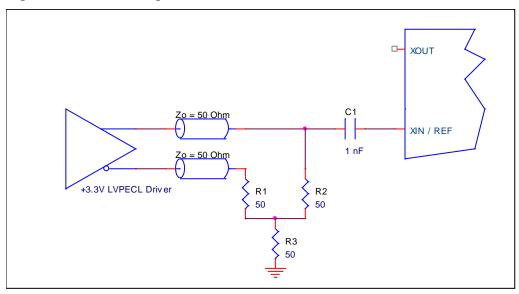
Table 23 shows resistor values that ensure the maximum drive level for the XIN port is not exceeded for all combinations of 5% tolerance on the driver  $V_{DD}$ ,  $V_{DDO0}$ , and 5% resistor tolerances. The resistor values can be adjusted to reduce the loading for a slower and weaker LVCMOS driver by increasing the impedance of the R1–R2 divider. To better assist with this assessment, the total load (Ro+Rs+R1+R2) on the driver is included in the table.
