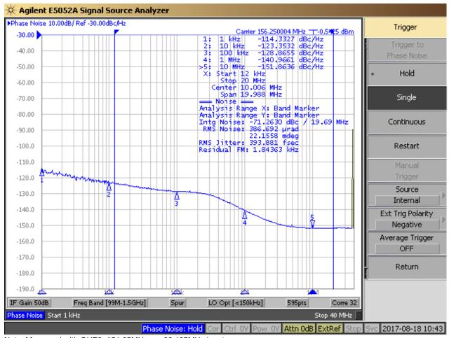
Note: Measured with OUT2=156.25MHz on, 39.625MHz input.
