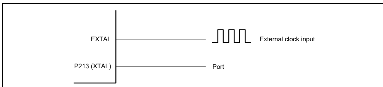
Figure 9.8 Equivalent circuit for external clock
