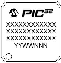
144-Lead TQFP (16x16x1 mm)
