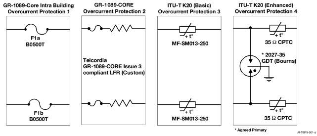
**Figure 5. Typical Overcurrent Protection**
