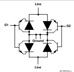
to provide independent control for each protection element. The gate buffer transistors minimize supply regulation issues by reducing the gate current drawn to around 5 mA, while the high voltage base emitter structures eliminate the need for expensive reverse bias protection gate diodes.
