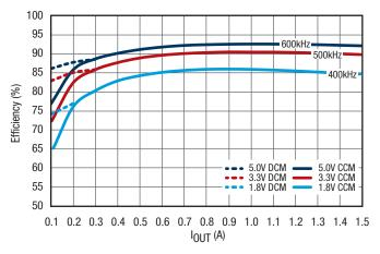
Figure 19. Efficiency,  $V_{IN} = 12V$
