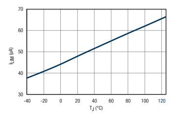
Figure 10. I<sub>LIM</sub> vs. Temperature
