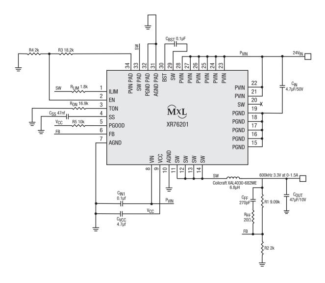
Figure 24. Application Circuit
