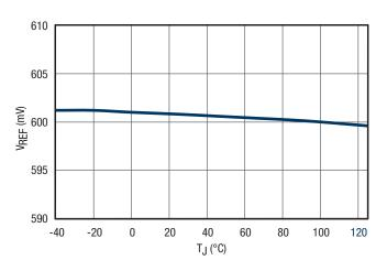
Figure 11. V<sub>REF</sub> vs. Temperature
