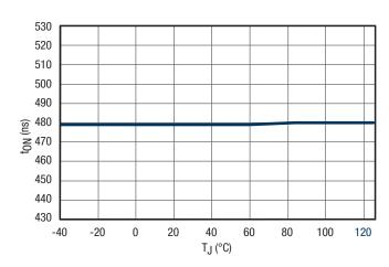
Figure 12.  $t_{ON}$  vs. Temperature,  $R_{ON} = 35.7 k\Omega$
