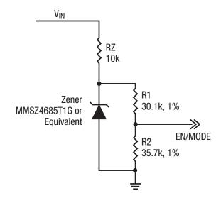
$\label{eq:Figure 22.} Figure 22.$  Selecting Forced CCM by Deriving EN/MODE from  $V_{\text{IN}}$
