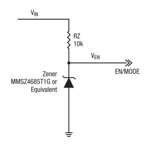
Figure 23. Selecting DCM/CCM by Deriving EN/MODE from  $V_{IN}$
