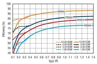
Figure 20. Efficiency,  $V_{IN} = 24V$
