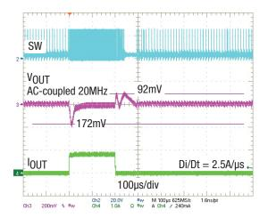
Figure 18. Load Step, DCM / CCM, 0.05A - 0.85A
