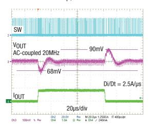
Figure 17. Load Step, Forced CCM, 0A - 0.8A
