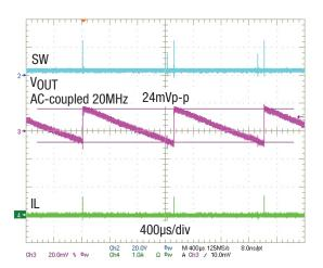
Figure 14. Steady State, DCM, I<sub>OUT</sub> = 0A
