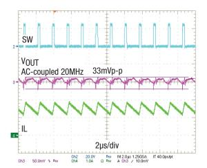
Figure 13. Steady State,  $I_{OUT} = 1.5A$
