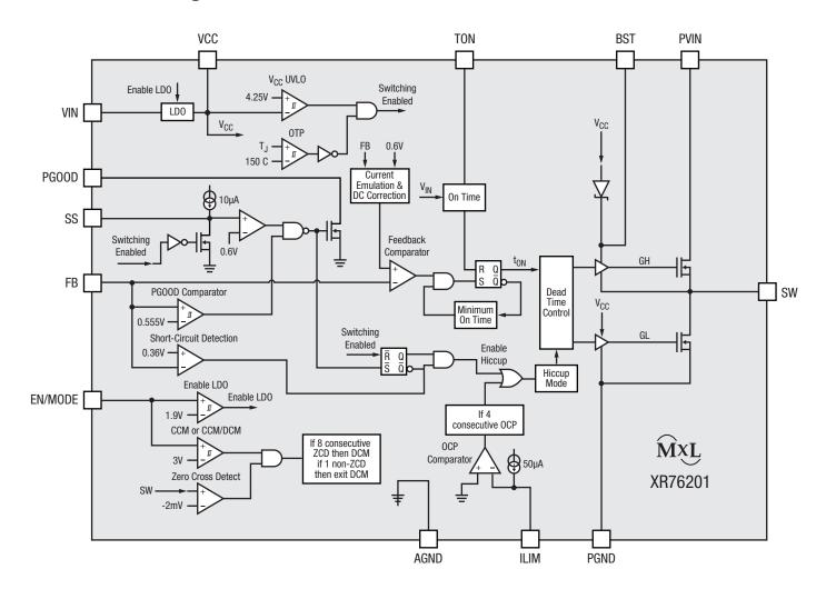
Figure 21. Functional Block Diagram
