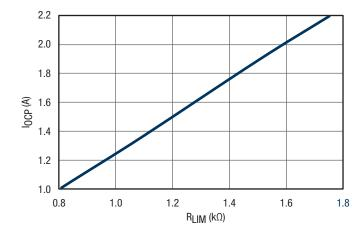
Figure 9. I<sub>OCP</sub> vs. R<sub>LIM</sub>
