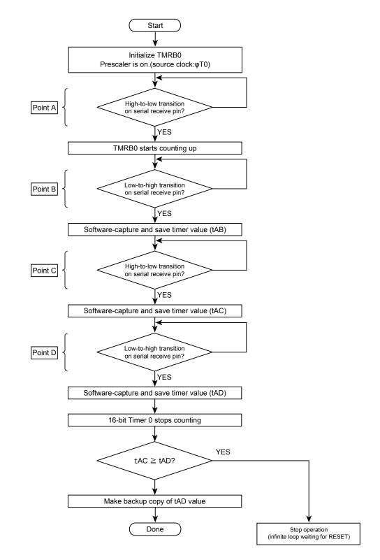
Figure 20-7 Serial operation mode receive flowchart
