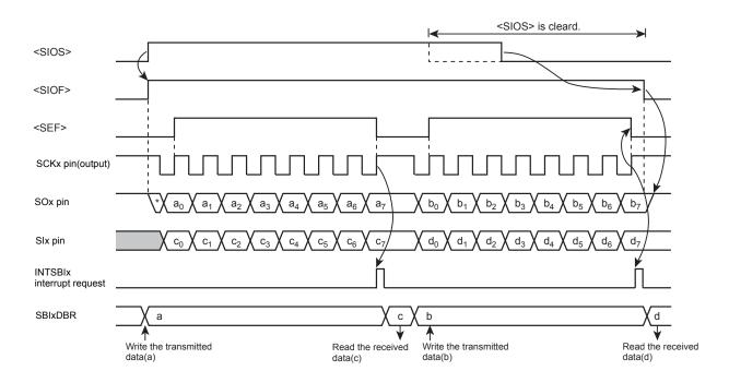
Figure 12-18 Transmit/Receive Mode (Example: Internal Clock)
