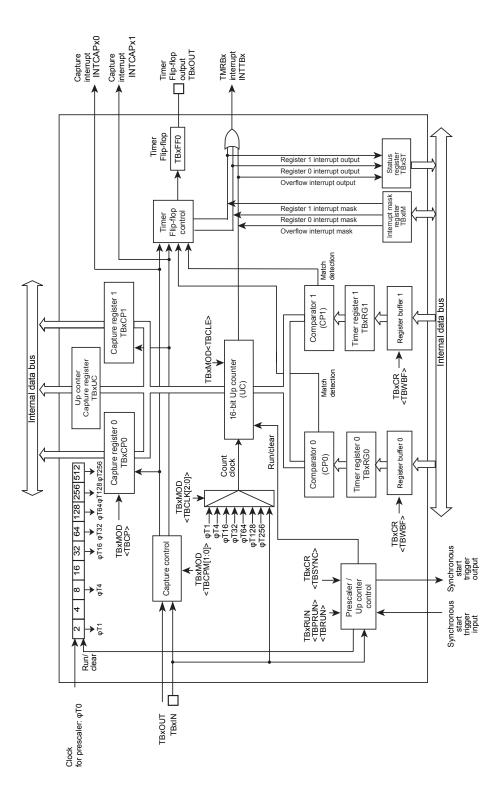
Figure 9-1 TMRBx Block Diagram
