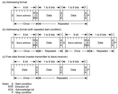
Figure 12-2 I2C Bus Mode Data Formats
