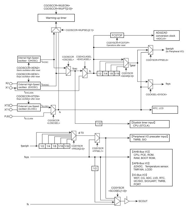
Figure 6-1 Clock Block Diagram
