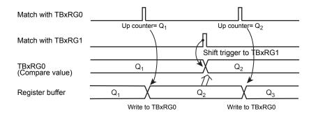
Figure 9-3 Register Buffer Operation
