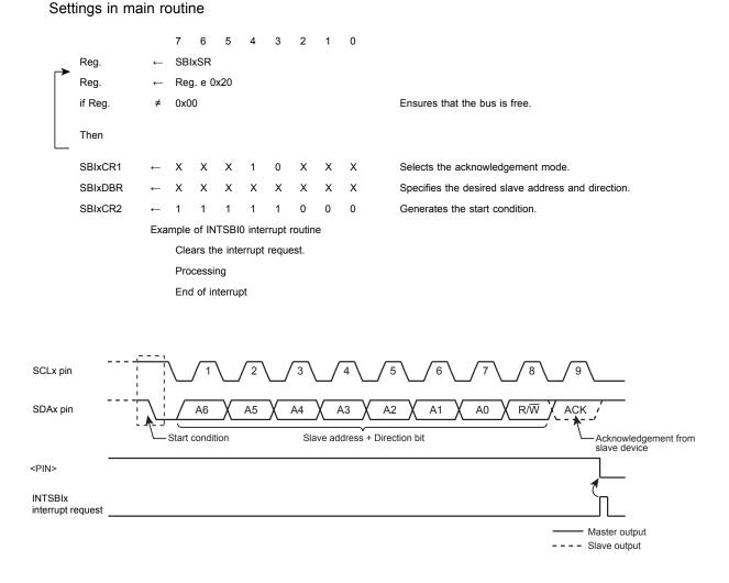
Figure 12-7 Generation of the Start Condition and a Slave Address
