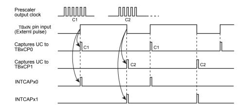
Figure 9-7 Pulse width measurement
