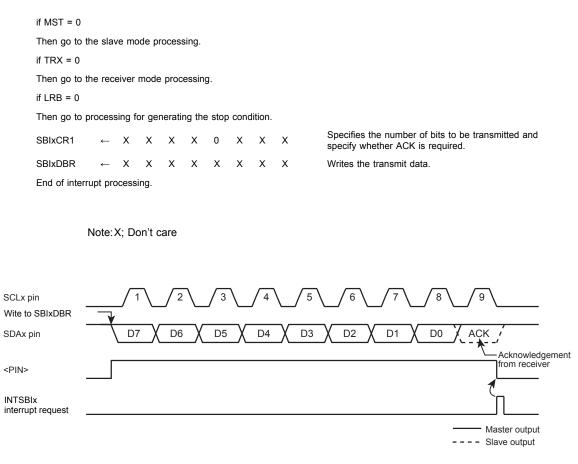
Figure 12-8 <BC[2:0]>= "000",<ACK>= "1" (Transmitter Mode)
