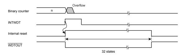
Figure 19-3 Internal reset generation
