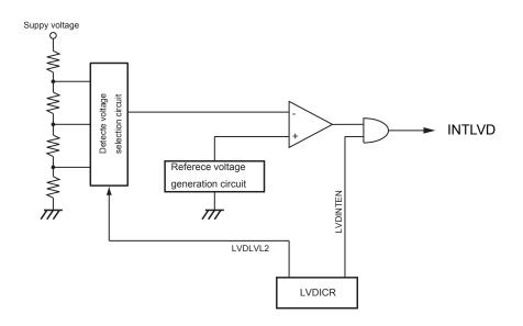
Figure 18-1 Block diagram of LVD (described only LVD interrupt circuit)
