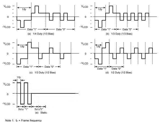
Note 2:  $V_{LCD3}$  = LCD drive voltage ( =  $V_{LC} - V_{SS}$ )
