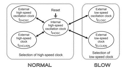
Figure 6-2 System clock switching
