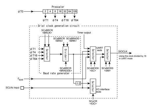
Figure 11-3 Serial clock generation circuit
