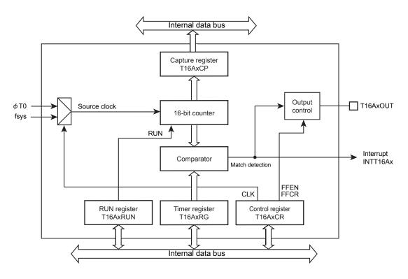
Figure 10-1 Block diagram of TMR16A
