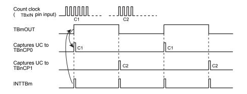
Figure 9-6 Frequency measurement
