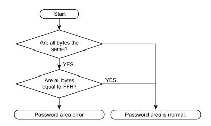
Figure 20-9 Password area check flowchart
