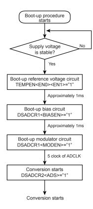
Figure 14-2 Boot-up procedure
