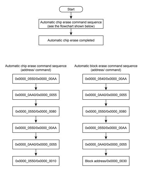
Figure 20-5 Flowchart of automatic erase
