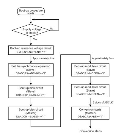
Figure 14-4 Synchronous start function procedure
