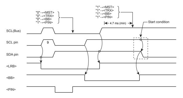
Figure 12-12 Timing Chart of Generating a Restart
