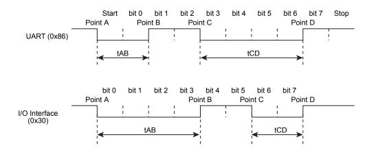
Figure 20-6 Serial operation mode determination data
