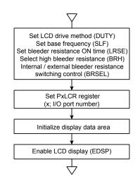
Figure 17-5 Flowchart for the LCD Driver Initialization
