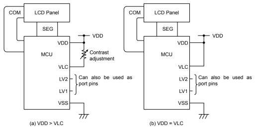
When internal bleeder resistance is used (LCDCR2<BRSEL>="1")
