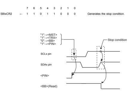
Figure 12-11 Generating the Stop Condition
