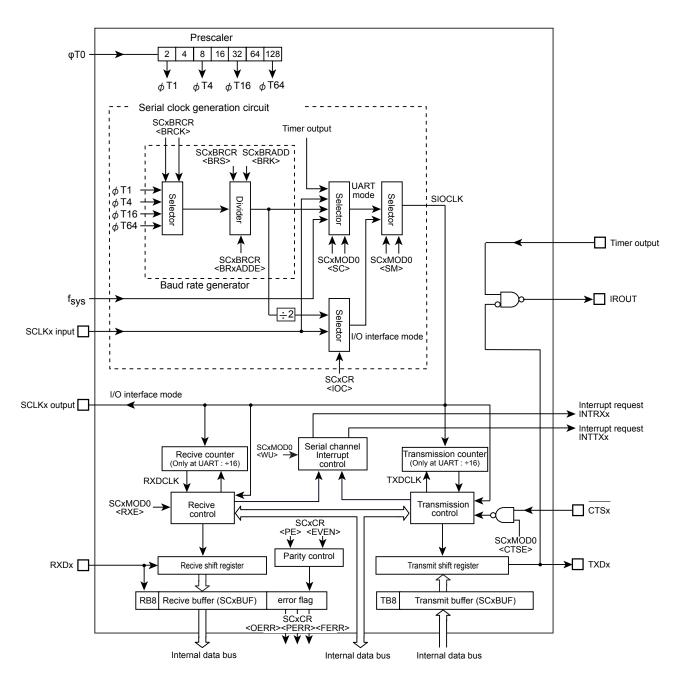
Figure 11-1 Serial Channel Block Diagram
