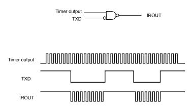
Figure 11-10 Output signal using IR carrier pulse
