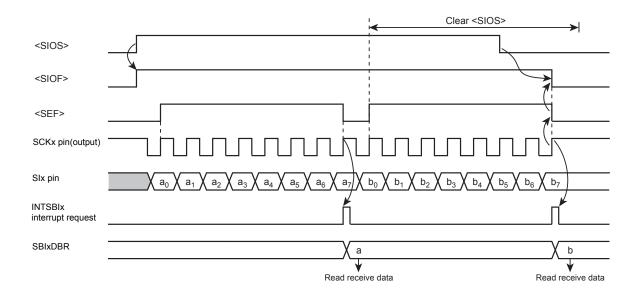
Figure 12-17 Receive Mode (Example: Internal Clock)
