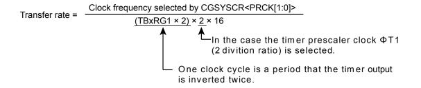
To enable the TMR16A output, a timer output inverts when the value of the counter and that of T16AxRG match. The SIOCLK clock frequency is "Setting value of T16AxRG  $\times$  2".
