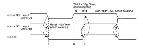
Figure 12-4 Example of Clock Synchronization
