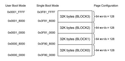
Figure 20-1 Block configuration
