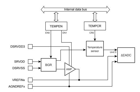
Figure 15-1 Block diagram of Temperature sensor
