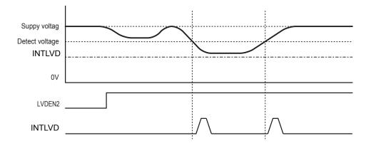
Figure 18-2 low voltage detection Timing
