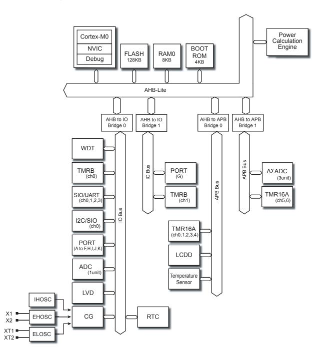
Figure 1-1 Block Diagram
