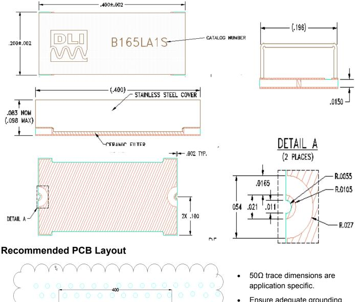
• Ensure adequate grounding beneath the part.
