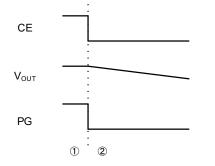
①The initial conditions, V<sub>OUT</sub> is a stable state. Assume C<sub>L</sub> high speed Discharge is activated by using MODE3 pin.
