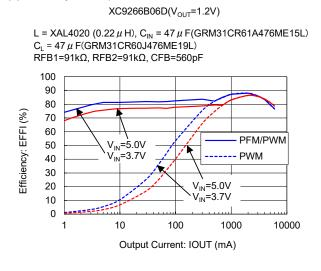
(1) Efficiency vs. Output Current
