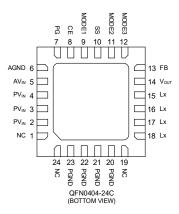
\* The dissipation pad for the QFN0404-24C package should be solder-plated in recommended mount pattern and metal masking so as to enhance mounting strength and heat release. If the pad needs to be connected to other pins, it should be connected to the GND (No. 6,20,21,22,23) pin.
