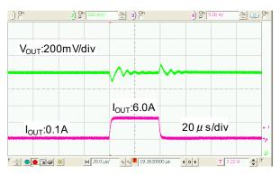
XC9266B06C V<sub>IN</sub>=5.0V V<sub>OUT</sub> = 1.2V f<sub>OSC</sub> = 1.2MHz l<sub>OUT</sub> = 0.1A ⇒ 6.0A L = XAL6030 (0.56μH), C<sub>IN</sub> = 47 μ F(GRM31CR61A476ME15L) C<sub>L</sub> = 47 μ F(GRM31CR60J476ME19L) RFB1=91kΩ, RFB2=91kΩ, CFB=560pF MODE1=L (PFWPWM)
