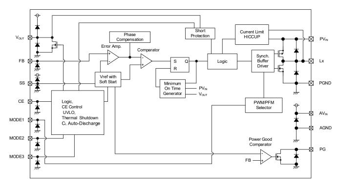
\* Diodes inside the circuit are an ESD protection diode and a parasitic diode.
