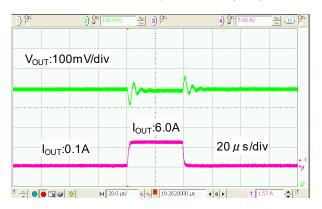
$\begin{array}{l} XC9266B06D \\ V_{\text{IN}} = 5.0V V_{\text{OUT}} = 1.2V f_{\text{OSC}} = 3.0 \text{MHz} I_{\text{OUT}} = 0.1 \text{A} \Rightarrow 6.0 \text{A} \\ L = XAL4020 (0.22 \, \mu \text{ H}), C_{\text{IN}} = 47 \, \mu \, \text{F}(\text{GRM31CR61A476ME15L}) \\ C_{\text{L}} = 47 \, \mu \, \text{F}(\text{GRM31CR60J476ME19L}) \\ \text{RFB1=91k}\Omega, \, \text{RFB2=91k}\Omega, \, \text{CFB=560pF} \, \text{MODE1=L} \, \left(\text{PFM/PWM}\right) \end{array}$
