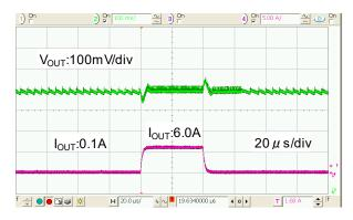
$\begin{array}{l} XC9266B06D \\ V_{\text{IN}} = 5.0V \ V_{\text{OUT}} = 1.8V \ f_{\text{OSC}} = 3.0\text{MHz} \ l_{\text{OUT}} = 0.1\text{A} \Rightarrow 6.0\text{A} \\ L = XAL4020 \ (0.22 \ \mu \ \text{H}), \ C_{\text{IN}} = 47 \ \mu \ \text{F}(\text{GRM31CR61A476ME15L}) \\ C_{\text{L}} = 47 \ \mu \ \text{F}(\text{GRM31CR60J476ME19L}) \\ \text{RFB1=36k}\Omega, \ \text{RFB2=18k}\Omega, \ \text{CFB=1500pF} \ \text{MODE1=L} \ (\text{PFWPWM}) \end{array}$
