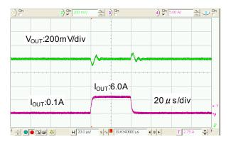
$\begin{array}{l} XC9266B06C \\ V_{\text{IN}} = 5.0V \ V_{\text{OUT}} = 3.3V \ f_{\text{SOC}} = 1.2 \text{MHz} \ l_{\text{OUT}} = 0.1 \text{A} \Rightarrow 6.0 \text{A} \\ L = XAL6030 \ (0.56 \mu\text{H}), \ C_{\text{IN}} = 47 \mu\text{F}(\text{GRM31CR61A476ME15L}) \\ C_{\text{L}} = 94 \mu\text{F}(\text{GRM31CR60J476ME19Lx2}) \\ \text{RFB1=68k}\Omega, \ \text{RFB2=15k}\Omega, \ \text{CFB=820pF} \ \text{MODE1=H} \ (\text{PWM}) \end{array}$
