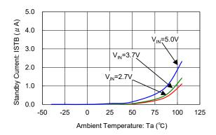
$\label{eq:constraint} \begin{array}{l} XC9266B06C \\ L = XAL6030 \mbox{ (}0.56 \mbox{ $\mu$ H)$, $C_{IN}$ = 47 \mbox{ $\mu$ F}$ (GRM31CR61A476ME15L) } \\ C_L = 47 \mbox{ $\mu$ F}$ (GRM31CR60J476ME19L) \\ RFB1=36k\Omega, $RFB2=18k\Omega, $CFB=1500pF $ MODE1=H (PWM)$ } \end{array}$
