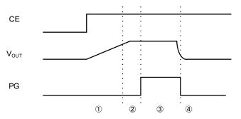
①Assume V<sub>IN</sub> has been applied.When H level is fed to the CE pin, V<sub>OUT</sub> will rise by using a Soft-start function. PG voltage is the GND level during Soft-start operation.
