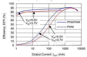
$$\label{eq:constraint} \begin{split} & \text{XC9266B06D}(\text{V}_{\text{OUT}}=3.3\text{V}) \\ \text{L} = \text{XAL4020} \ (0.22 \ \mu \ \text{H}), \ \text{C}_{\text{IN}} = 47 \ \mu \ \text{F}(\text{GRM31CR61A476ME15L}) \\ \text{C}_{\text{L}} = 94 \ \mu \ \text{F}(\text{GRM31CR60J476ME19Lx2}) \\ \text{RFB1=68k}\Omega, \ \text{RFB2=15}\Omega, \ \text{CFB=820pF} \end{split}$$
