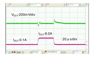
$\begin{array}{l} XC9266B06C \\ V_{\text{IN}} = 5.0V \; V_{\text{OUT}} = 3.3V \; f_{\text{OSC}} = 1.2 \text{MHz} \; l_{\text{OUT}} = 0.1 \text{A} \Rightarrow 6.0 \text{A} \\ \text{L} = XAL6030 \; (0.56 \mu\text{H}), \; C_{\text{IN}} = 47 \mu\text{F}(\text{GRM31CR61A476ME15L}) \\ C_{\text{L}} = 94 \mu\text{F}(\text{GRM31CR60J476ME19Lx2}) \\ \text{RFB1=68k}\Omega, \; \text{RFB2=15k}\Omega, \; \text{CFB=820pF} \; \text{MODE1=L} \; (\text{PFM/PWM}) \end{array}$
