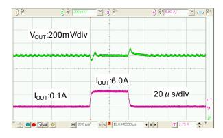
XC9266B06C V<sub>IN</sub> = 5.0V V<sub>OUT</sub> = 1.8V f<sub>OSC</sub> = 1.2MHz I<sub>OUT</sub> = 0.1A ⇒ 6.0A L = XAL6030 (0.56µH), C<sub>IN</sub> = 47  $\mu$  F(GRM31CR61A476ME15L) C<sub>L</sub> = 47  $\mu$  F(GRM31CR60J476ME19L) RFB1=36kΩ, RFB2=18kΩ, CFB=1500pF MODE1=L (PFM/PWM)
