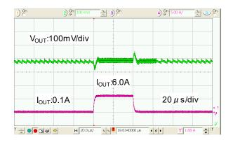
XC9266B06D  $V_{IN}$ =5.0V  $V_{OUT}$ = 3.3V  $f_{OSC}$ =3.0MHz  $I_{OUT}$ = 0.1A ⇒ 6.0A L = XAL4020 (0.22µH),  $C_{IN}$  = 47µF(GRM31CR61A476ME15L) CL = 94µF(GRM31CR60J476ME19Lx2) EFE4 60420 EFE02 45120 CFE0 2020 F MODE4 + (PEM/EM/
