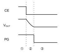
① The initial conditions,  $V_{OUT}$  is a stable state. Assume Soft-off function is activated by using MODE3 pin. ②L level is fed to CE pin and then XC9266 is in a standby state. Therefore  $V_{OUT}$  begins to fall down sharply by soft-off function. In this case, PG voltage goes down to GND level ( $V_{OUT} = 0.2V$  or less) after soft-off function is completed.
