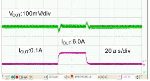
XC9266B06D V<sub>IN</sub>=5.0V V<sub>OUT</sub> = 1.8V f<sub>OSC</sub> = 3.0MHz I<sub>OUT</sub> = 0.1A ⇒ 6.0A L = XAL4020 (0.22 μ H), C<sub>IN</sub> = 47 μ F(GRM31CR61A476ME15L) C<sub>L</sub> = 47 μ F(GRM31CR60J476ME19L) RFB1=36kΩ, RFB2=18kΩ, CFB=1500pF MODE1=H (PWM)
