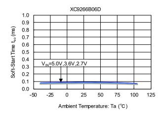
(23)Soft-Start Time vs. Ambient Temperature
