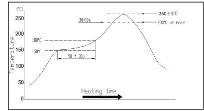
Temperature profile for reflow soldering
