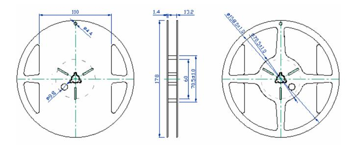
1.230mm minimum leafer which consist of carrier and/or tape followed by a minimum of 160mm of empty carrier tape sealed with cover tape.
