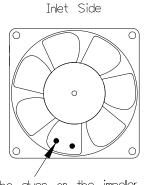
Note: The glues on the impeller is for impeller balance.
