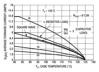
Figure 6. Current Derating, Infinite Heatsink
