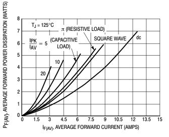
Figure 9. Forward Power Dissipation
