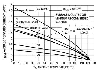
Figure 8. Current Derating, Free Air
