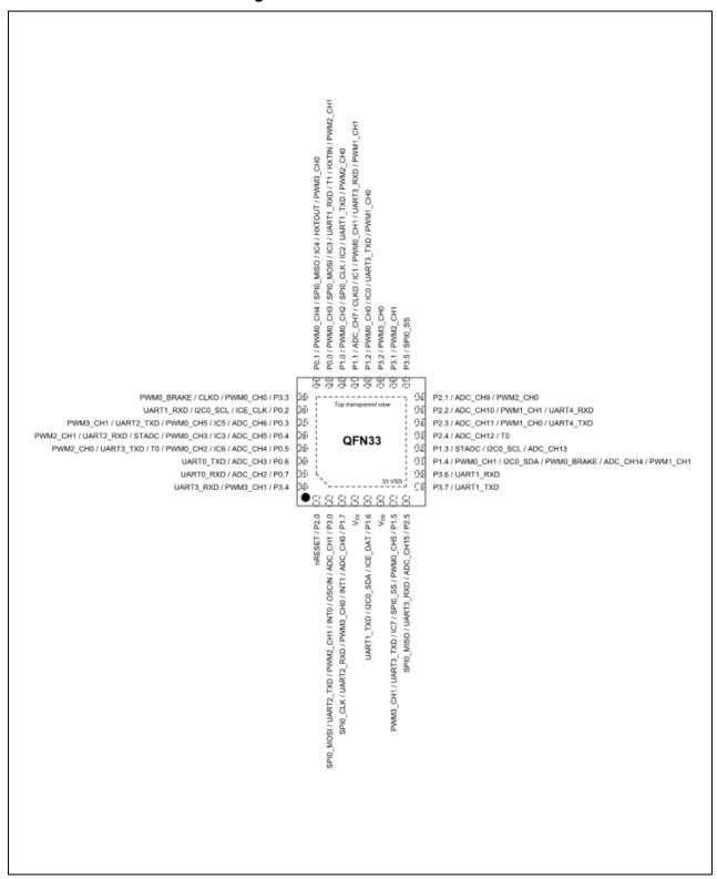
Figure 5-2 MS51 Series QFN-33 -pin Diagram
