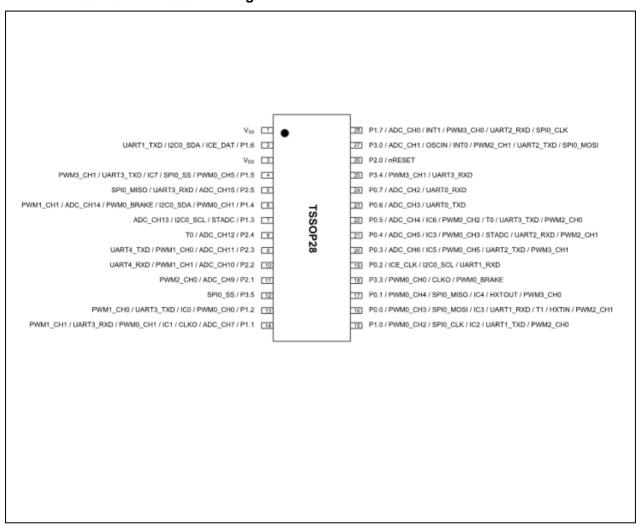
Figure 5-3 MS51 Series TSSOP-28 -pin Diagram
