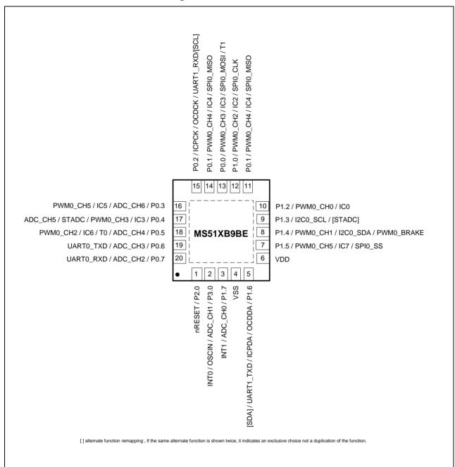
Figure 5-7 MS51 Series QFN-20-pin Diagram
