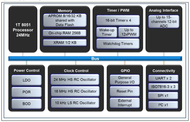
Figure 3-1 NuMicro® MS51 Block Diagram
