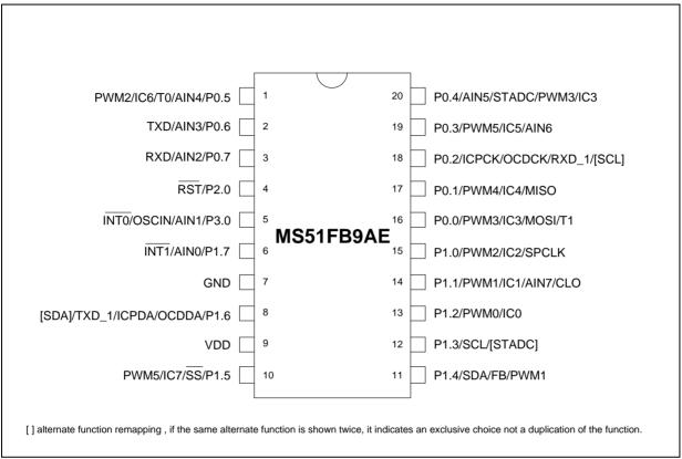
Figure 5-6 MS51 Series TSSOP-20 -pin Diagram
