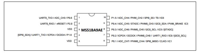
Figure 5-10 MS51 Series MSOP-10-pin Diagram
