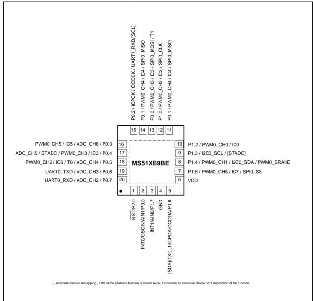
Figure 5-8 MS51 Series QFN-20-pin Diagram
