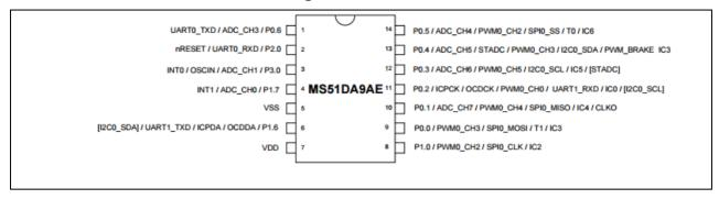
Figure 5-9 MS51 Series TSSOP-14-pin Diagram
