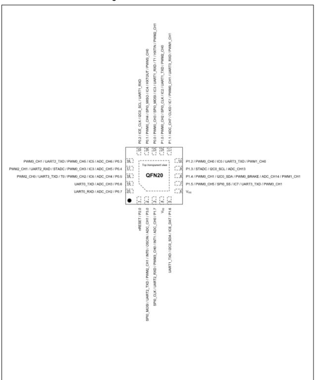
Figure 5-5 MS51 Series QFN-20 -pin Diagram
