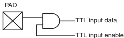
Figure 1.3 (2) Simplified Circuit Diagram (TTL AND Input Buffer)
