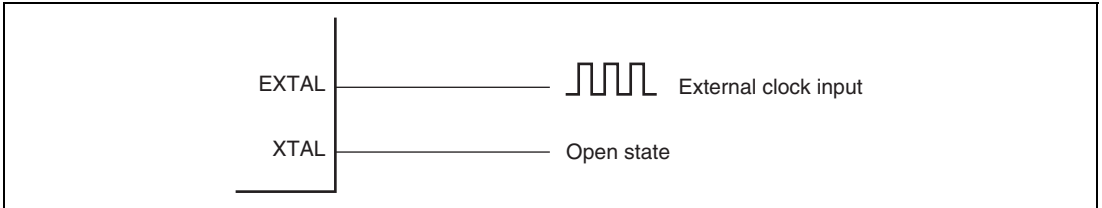
Figure 4.4 Example of External Clock Connection
