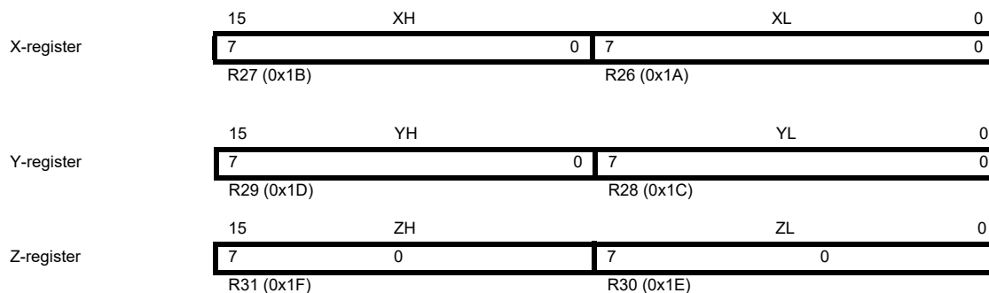
Figure 7-3. The X-, Y-, and Z-registers
