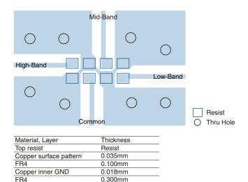
$\begin{tabular}{ll} \hline Copper bottom GND & 0.035mm \\ \hline Line width should be designed to match <math>50\Omega$  characteristic impedance, depending on PCB material and thickness. \\ \hline \end{tabular}
