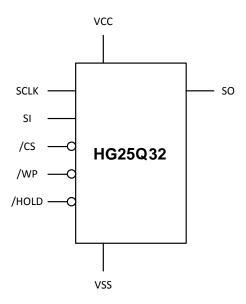
Figure 2. Pin Configuration SOP8L/DIP8L
