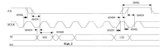
Figure 37. Output Timing
