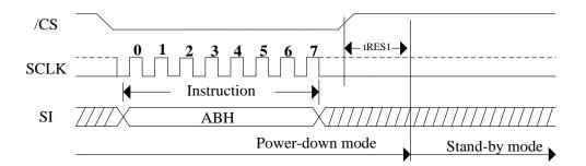
Figure 23b. Release Power-Down/Read Device ID Sequence Diagram
