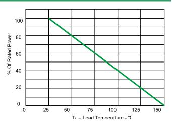
Fig 2.Power Derating Curve
