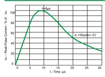
Fig 1.Pulse Waveform
