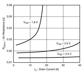
On-Resistance vs. Drain Current and Gate Voltage
