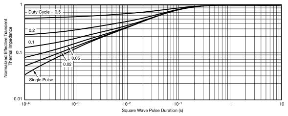
Normalized Thermal Transient Impedance, Junction-to-Foot
