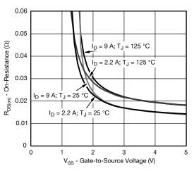
On-Resistance vs. Gate-to-Source Voltage
