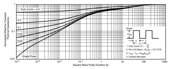
Normalized Thermal Transient Impedance, Junction-to-Ambient
