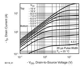
Fig. 1 - Typical Output Characteristics, T<sub>C</sub> = 25 °C
