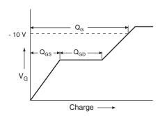
Fig. 13a - Basic Gate Charge Waveform
