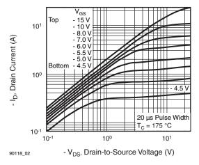
Fig. 2 - Typical Output Characteristics,  $T_C$  = 175  $^{\circ}$  C
