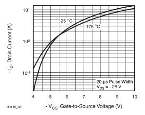
Fig. 3 - Typical Transfer Characteristics
