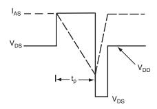
Fig. 12b - Unclamped Inductive Waveforms
