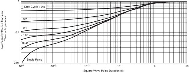
Normalized Thermal Transient Impedance, Junction-to-Foot
