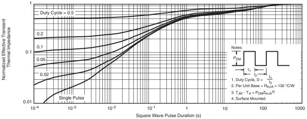
Normalized Thermal Transient Impedance, Junction-to-Ambient
