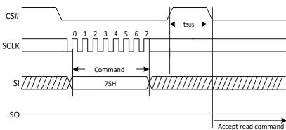
Figure 40. Program/Erase Suspend Sequence Diagram
