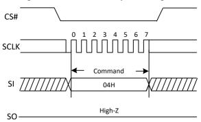
Figure 5a. Write Disable Sequence Diagram (QPI)
