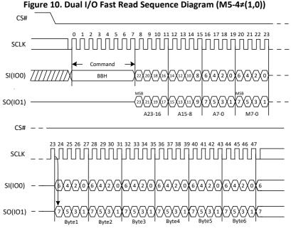
Dual I/O Fast Read with "Continuous Read Mode"
