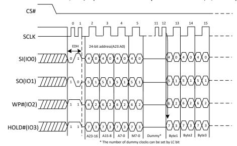
Figure 17b. DTR Fast Read Quad I/O (Initial instruction or previous M5-4≠10, QPI Mode)
