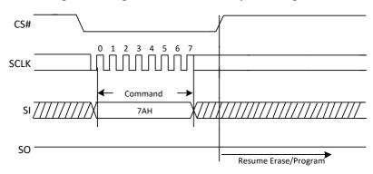
Figure 41. Program/Erase Resume Sequence Diagram
