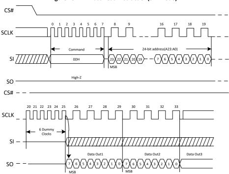
Figure 15. DTR Fast Read Instruction(SPI Mode)
