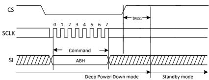
Figure 30. Release Power-Down Sequence Diagram
