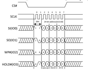
Figure 38d. Read Individual Block/Sector lock command Sequence Diagram
