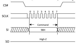
Figure 39c. The Global Block/Sector Unlock Sequence Diagram (QPI)
