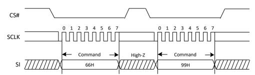
Figure 31. Enable Reset and Reset command Sequence Diagram
