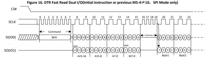
DTR Fast Read Dual I/O with "Continuous Read Mode"
