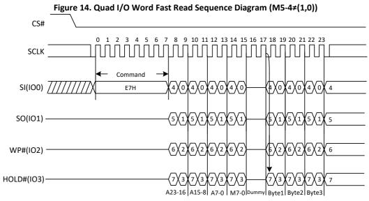
Quad I/O Word Fast Read with "Continuous Read Mode"
