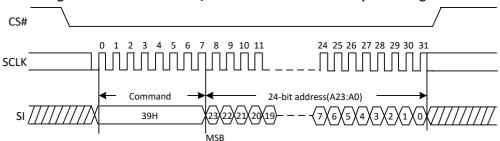
Figure 38c. Individual Block/Sector Unlock command Sequence Diagram (QPI)
