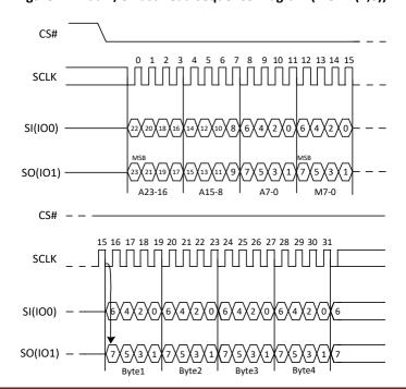
Figure 11. Dual I/O Fast Read Sequence Diagram (M5-4=(1,0))
