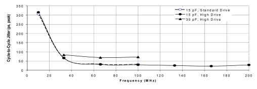
Figure 14. Typical 3.3 V Measured Period Jitter at 29 °C, versus Frequency, Drive Strength, and Loading
