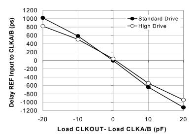
Data is shown for 66 MHz. Delay is a weak function of frequency.
