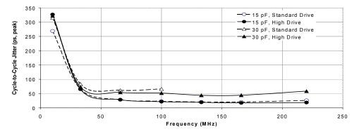
Figure 12. Typical 3.3 V Measured Cycle-to-cycle Jitter at 29 °C, versus Frequency, Drive Strength, and Loading
