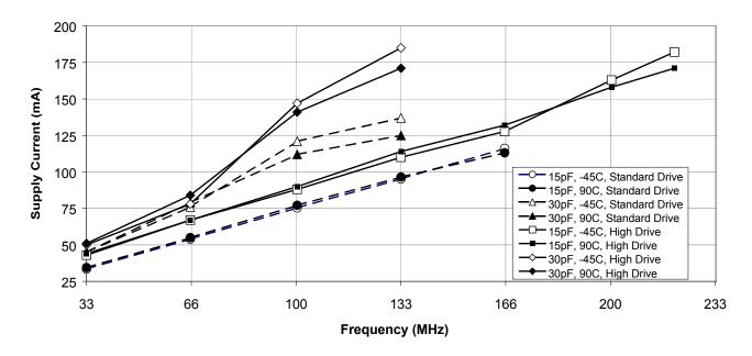
Figure 10. 3.6 V Measured Supply Current versus Frequency, Drive Strength, Loading, and Temperature
