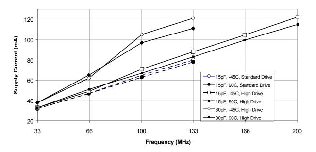
Note that the 30-pF high-drive data above 100bMHz is beyond the data sheet specification of 22 pF.
