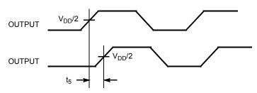
Figure 6. Input-Output Propagation Delay
