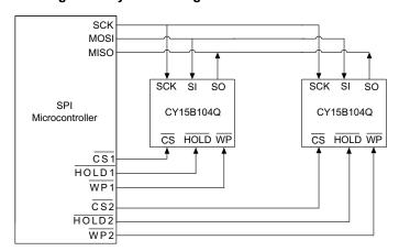
Figure 3. System Configuration with SPI Port
