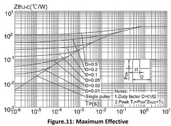
Transient Thermal Impedance, Junction-to-Case
