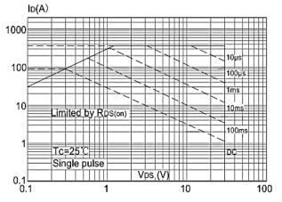
Figure 9: Maximum Safe Operating Area vs. Case Temperature
