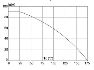
Figure 10: Maximum Continuous Drain Current
