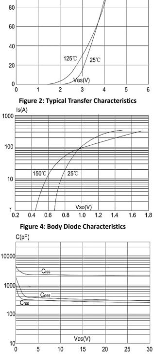
Figure 6: Capacitance Characteristics
