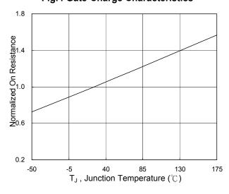
Fig.6 Normalized R<sub>DSON</sub> vs. T<sub>J</sub>
