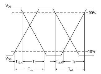
Fig.10 Switching Time Waveform
