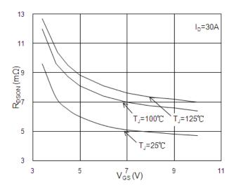
Fig.2 On-Resistance vs. G-S Voltage
