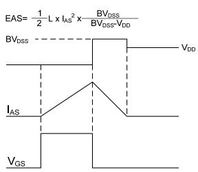
Fig.11 Unclamped Inductive Switching Waveform
