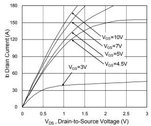
Fig.1 Typical Output Characteristics
