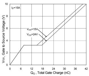
Fig.4 Gate-Charge Characteristics
