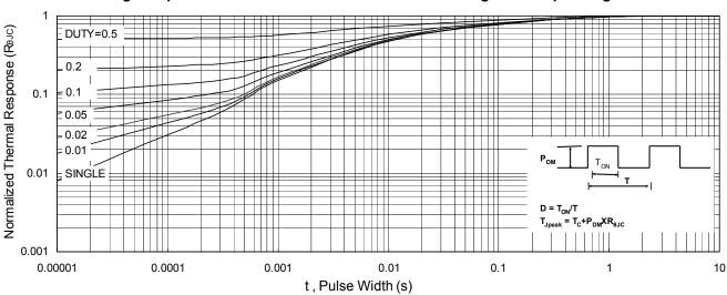
Fig.9 Normalized Maximum Transient Thermal Impedance
