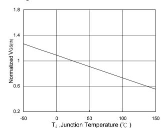
Fig.5 Normalized  $V_{GS(th)}$  vs.  $T_J$
