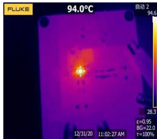
Figure 22. Thermal, 12 VIN, 1 Vout, 5A
