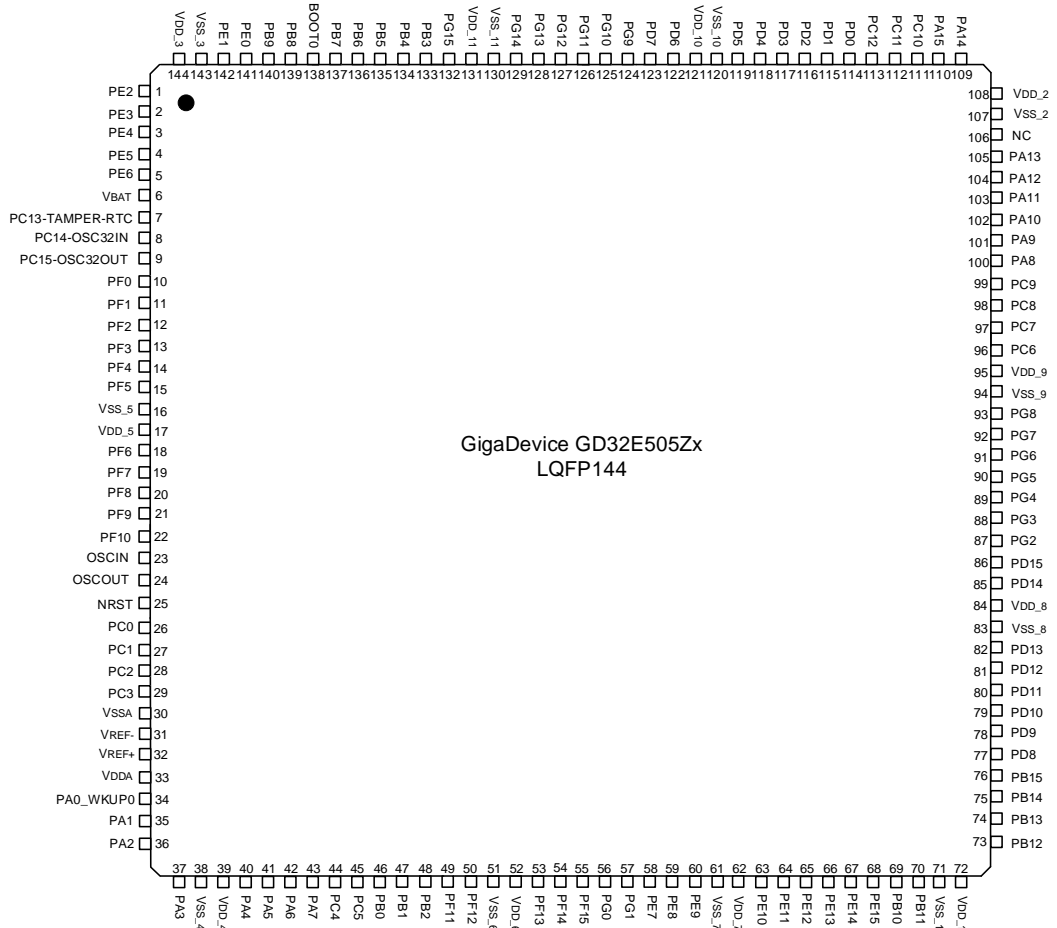
Figure 2-2. GD32E505Zx LQFP144 pinouts
