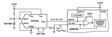
Figure 19. Single-Supply Gain Control Circuit
