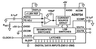
The AD9754 is a current-output DAC with a nominal full-scale output current of 20 mA and > 100 k $\Omega$  output impedance.
