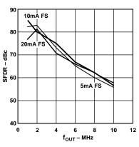
Figure 8. SFDR vs. f<sub>OUT</sub> and I<sub>OUTFS</sub> @ 25 MSPS and 0 dBFS
