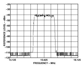
Figure 37. CDMA Signal, Sampled at 65 MSPS, Adjacent Channel Power >70 dB
