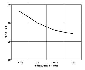
Figure 32. Power Supply Rejection Ratio of AD9754
