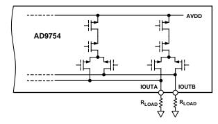
Figure 21. Equivalent Analog Output Circuit
