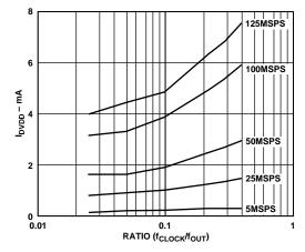
Figure 26.  $I_{DVDD}$  vs. Ratio @ DVDD = 3 V
