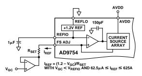
Figure 20. Dual-Supply Gain Control Circuit
