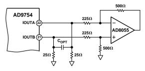
Figure 28. DC Differential Coupling Using an Op Amp
