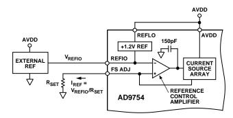
Figure 18. External Reference Configuration
