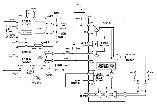
Figure 36. CDMA Transmit Application Using AD9754
