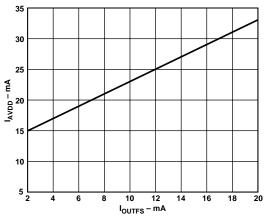
Figure 24. I<sub>AVDD</sub> vs. I<sub>OUTFS</sub>
