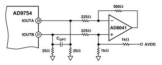
Figure 29. Single-Supply DC Differential Coupled Circuit
