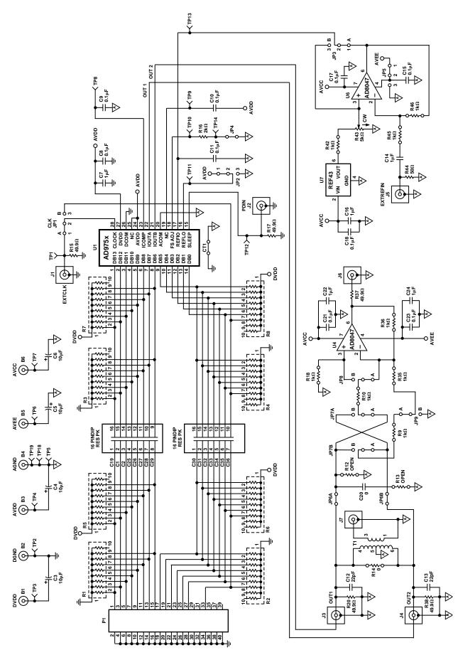
Figure 38. Evaluation Board Schematic
