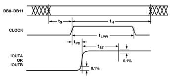
Figure 1. Timing Diagram
