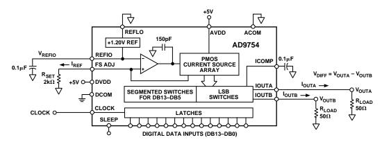
Figure 16. Functional Block Diagram
