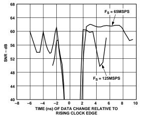
Figure 23. SNR vs. Clock Placement @  $f_{OUT}$  = 10 MHz
