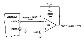
Figure 31. Unipolar Buffered Voltage Output
