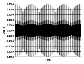
*Figure 34b. Time Domain "Snapshot" of the Multitone Waveform*
