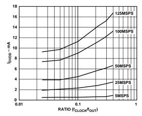
Figure 25. I<sub>DVDD</sub> vs. Ratio @ DVDD = 5 V
