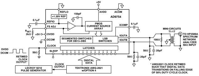
Figure 2. Basic AC Characterization Test Setup
