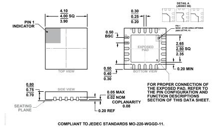
Figure 44. 20-Lead Frame Chip Scale Package [LFCSP] 4 mm × 4 mm Body and 0.75 mm Package Height (CP-20-10) Dimensions shown in millimeters
