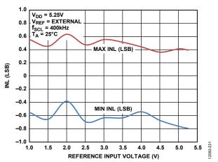
Figure 6. Minimum/Maximum INL vs. External Reference Input Voltage
