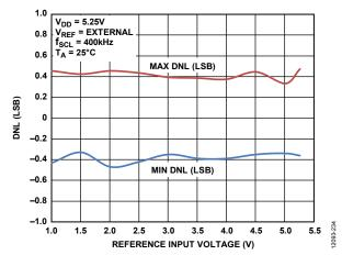
Figure 9. Minimum/Maximum DNL vs. External Reference Input Voltage
