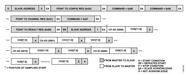
Figure 43. Command Mode Operation
