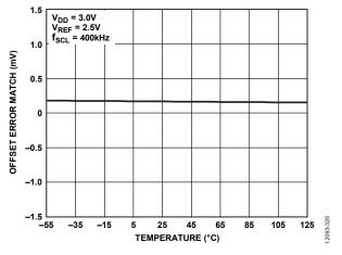
Figure 24. Offset Error Match vs. Temperature
