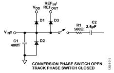
Figure 36. Equivalent Analog Input Circuit
