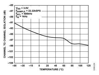
Figure 29. Channel to Channel Isolation vs. Temperature
