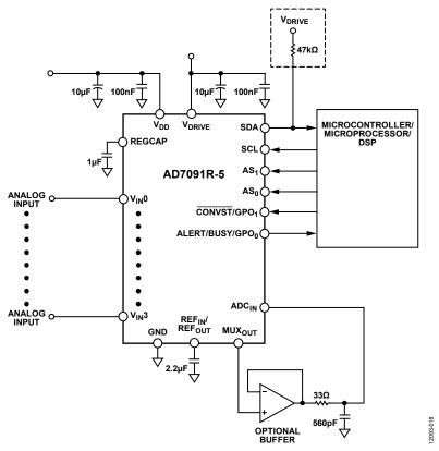
Figure 37. Typical Connection Diagram with Optional Buffer
