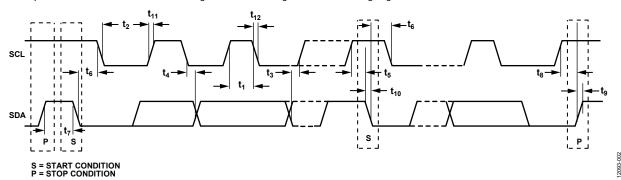
Figure 2. 2-Wire Serial Interface Timing Diagram
