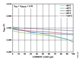
Figure 22. Reference Voltage Output (V<sub>REF</sub>) vs. Current Load for Various Temperatures
