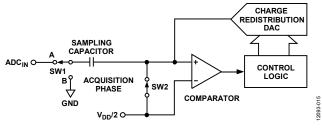
Figure 32. ADC Acquisition Phase
