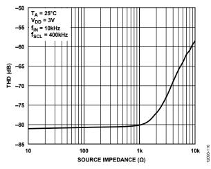
Figure 30. THD vs. Source Impedance
