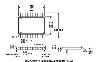
Figure 45. 20-Lead Thin Shrink Small Outline Package [TSSOP] (RU-20) Dimensions shown in millimeters
