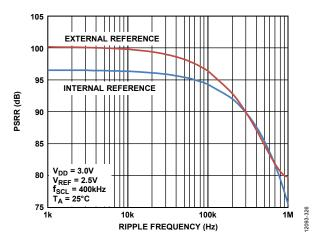
Figure 25. PSRR vs. Ripple Frequency
