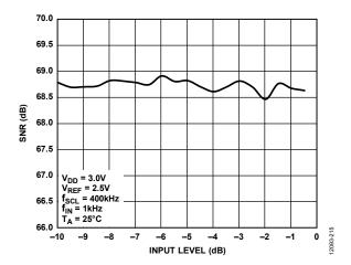
Figure 16. SNR vs. Input Level
