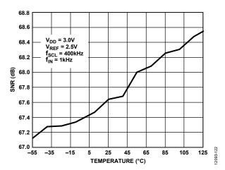
Figure 19. SNR vs. Temperature
