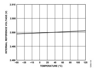
Figure 31. Internal Reference Voltage vs. Temperature
