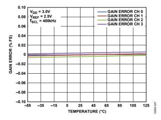
Figure 26. Gain Error vs. Temperature
