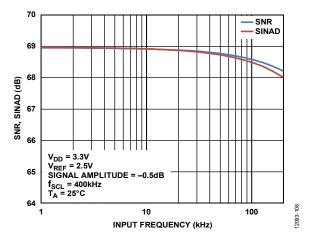
Figure 13. SNR, SINAD vs. Input Frequency
