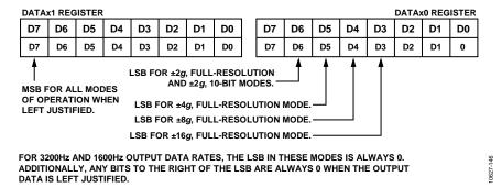
Figure 40. Data Formatting of Full-Resolution and  $\pm 2$  g, 10-Bit Modes of Operation When Output Data Is Left Justified
