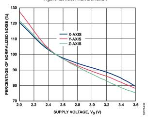
Figure 43. Normalized Noise vs. Supply Voltage,  $V_S$
