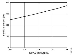
Figure 23. Supply Current vs. Supply Voltage,  $V_S$  at  $25^{\circ}C$
