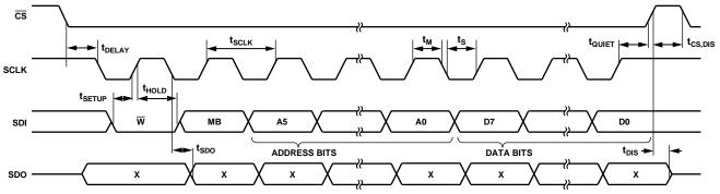
Figure 27. SPI 4-Wire Write
