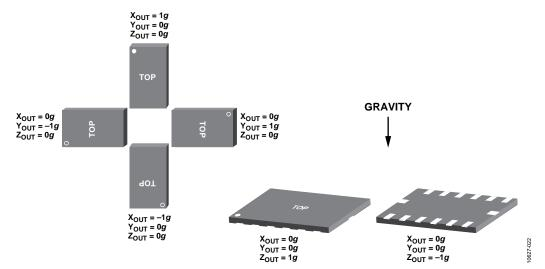
Figure 48. Output Response vs. Orientation to Gravity
