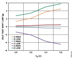
Figure 33. Self-Test Output Change Limits vs. Supply Voltage
