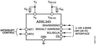
Figure 34. Application Diagram
