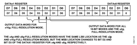
Figure 39. Data Formatting of Full-Resolution and  $\pm 2$  q, 10-Bit Modes of Operation When Output Data Is Right Justified
