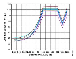
Figure 22. Current Consumption vs. Output Data Rate at 25°C—10 Parts,  $V_S = 2.5 \ V$
