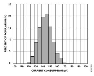
Figure 12. Current Consumption at 25°C, 100 Hz Output Data Rate,  $V_S = 2.5 \text{ V}$
