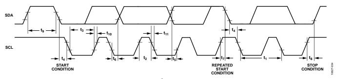
Figure 32. I<sup>2</sup>C Timing Diagram
