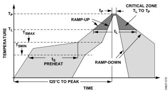
Figure 50. Recommended Soldering Profile
