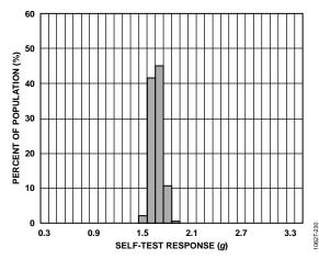
Figure 21. Z-Axis Self-Test Response at 25°C,  $V_S = 2.5 V$
