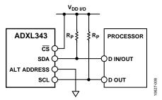
Figure 30. I<sup>2</sup>C Connection Diagram (Address 0x53)
