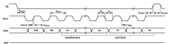
Figure 29. SPI 3-Wire Read/Write
