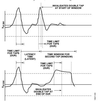
Figure 38. Tap Interrupt Function with Invalid Double Taps
