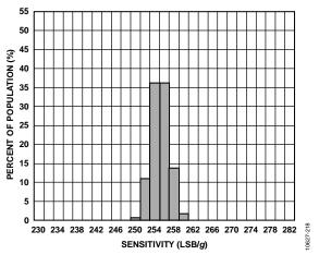
Figure 10. Sensitivity at 25°C,  $V_S = 2.5 V$ , Full Resolution, All Axes
