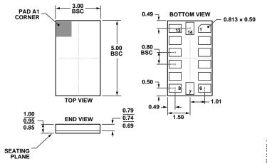
Figure 51. 14-Terminal Land Grid Array [LGA] (CC-14-1) Solder Terminations Finish Is Au over Ni Dimensions shown in millimeters
