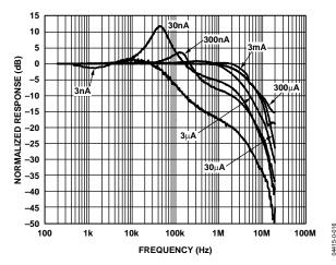
Figure 16. Small Signal AC Response,  $I_{REF}$  to  $V_{OUT}$  ( $A_V = 1$ ) (5% Sine Modulation, Decade Steps from 3 nA to 3 mA)
