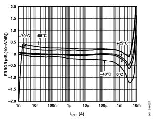
Figure 7. Law Conformance Error vs.  $I_{REF}$  for Multiple Temperatures, Normalized to 25°C ( $I_{INF} = 3 \mu A$ )
