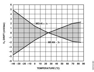
Figure 22. Slope Drift vs. Temperature (3 $\sigma$  to Either Side of Mean) Normalized to 25°C
