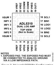
Figure 2. 24-Lead LFCSP Pin Configuration
