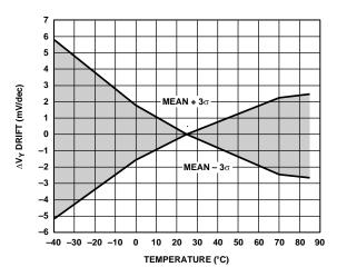
Figure 25. Slope Mismatch Drift vs. Temperature  $(V_{Y1} - V_{Y2}, 3\sigma \text{ to Either Side of Mean})$  Normalized to 25°C
