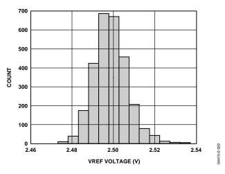
Figure 29. Distribution of  $V_{REF}$  ( $R_L = 100 \text{ k}\Omega$ )
