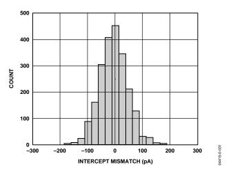
Figure 31. Distribution of Channel-to-Channel Intercept Mismatch ( $I_{Z1} - I_{Z2}$ )
