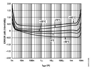
Figure 6. Law Conformance Error vs. I<sub>INP</sub> for Multiple Temperatures, Normalized to 25°C
