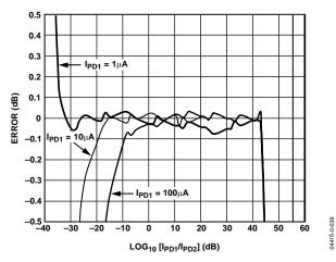
Figure 39. Log Conformance for Wilson Mirror ADL5310 Combination, Normalized to 10 mA Channel 1 Input Current, I<sub>№1</sub>
