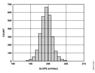
Figure 27. Distribution of Logarithmic Slope
