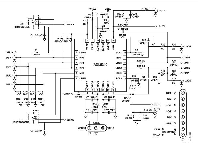
Figure 40. Evaluation Board Schematic
