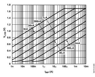
Figure 5. V<sub>LOG</sub> vs. I<sub>INP</sub> for Multiple Values of I<sub>REF</sub>, Decade Steps from 3 nA to 3 mA
