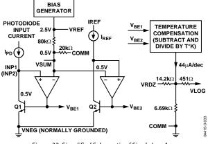
Figure 33. Simplified Schematic of Single Log Amp
