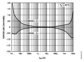
Figure 13. Law Conformance Error Distribution ( $3\sigma$  to Either Side of Mean)
