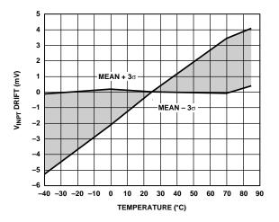
Figure 24. V<sub>INPT</sub> Drift vs. Temperature (3σ to Either Side of Mean) Normalized to 25°C
