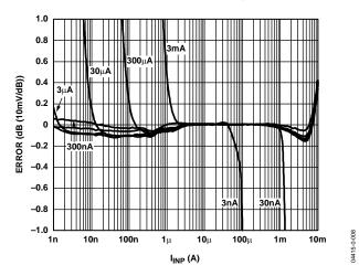
Figure 8. Law Conformance Error vs. I<sub>INP</sub> for Multiple Values of I<sub>REF</sub>, Decade Steps from 3 nA to 3 mA
