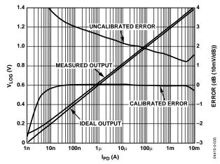
Figure 35. Using 2-Point Calibration to Increase Measurement Accuracy
