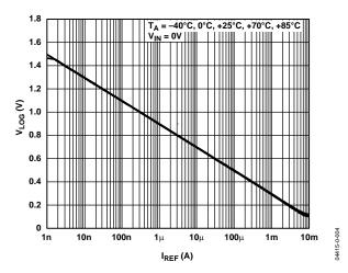
Figure 4.  $V_{LOG}$  vs.  $I_{REF}$  for Multiple Temperatures ( $I_{INP} = 3 \mu A$ )
