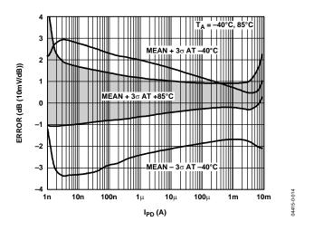
Figure 14. Law Conformance Error Distribution (3o to Either Side of Mean)
