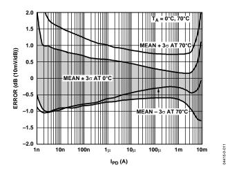
Figure 11. Law Conformance Error Distribution (3o to Either Side of Mean)
