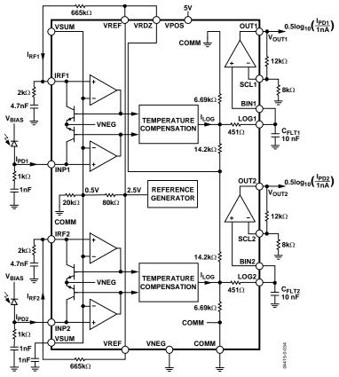
Figure 34. Basic Connections for Fixed Intercept Use
