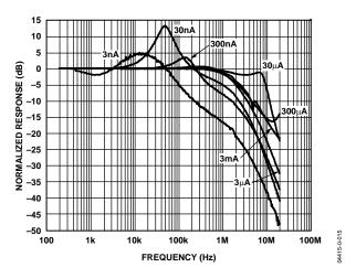
Figure 15. Small Signal AC Response,  $I_{INP}$  to  $V_{OUT}$  ( $A_V = 1$ ) (5% Sine Modulation, Decade Steps from 3 nA to 3 mA)
