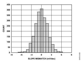
Figure 30. Distribution of Channel-to-Channel Slope Mismatch ( $V_{Y1} - V_{Y2}$ )
