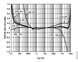
Figure 10. Law Conformance Error vs. IINP for Various Supply Conditions
