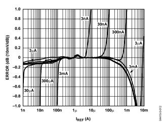
Figure 12. Law Conformance Error vs. IREE for Multiple Values of IINP, Decade Steps from 3 nA to 3 mA
