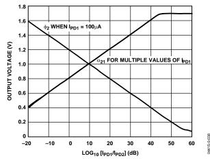
Figure 38. Absorbance and Absolute Power Transfer Functions for Wilson Mirror ADL5310 Combination
