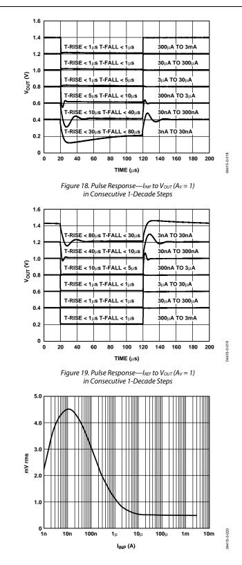
Figure 20. Total Wideband Noise Voltage at  $V_{OUT}$  vs.  $I_{INP}$  ( $A_V = 1$ )
