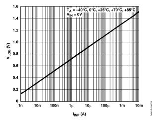
Figure 3. V<sub>LOG</sub> vs. I<sub>INP</sub> for Multiple Temperatures
