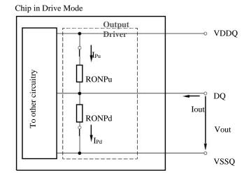
Figure 5.7 Output Driver : Definition of Voltages and Currents
