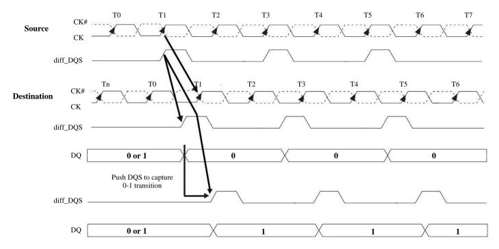
Figure 2.4.7 Write Leveling Concept
