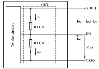
Figure 5.8.1 On-Die Termination : Definition of Voltages and Currents
