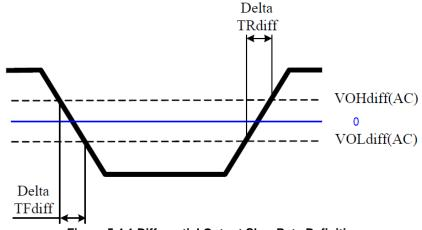
Figure 5.4.1 Differential Output Slew Rate Definition
