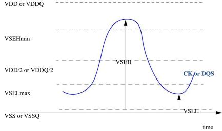
Figure 4.3.3 Single-ended requirement for differential signals.
