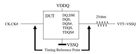
Figure 5.9.1 ODT Timing Reference Load
