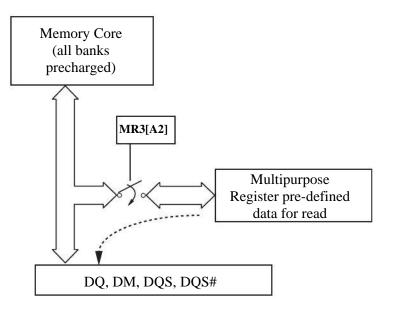
Figure 2.3.5.1 MPR Block Diagram
